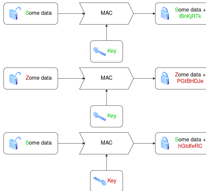
Figure 2.4: Basic concept of Message Authentication Codes (MACs). Small changes in input or key result in different hash.
