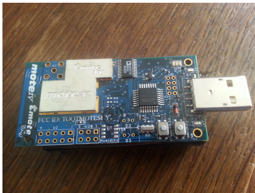
Figure 2.1: Tmote Sky MTM-CM5000-MSP battery powered wireless sensor node, using a TI MSP430 microcontroller
