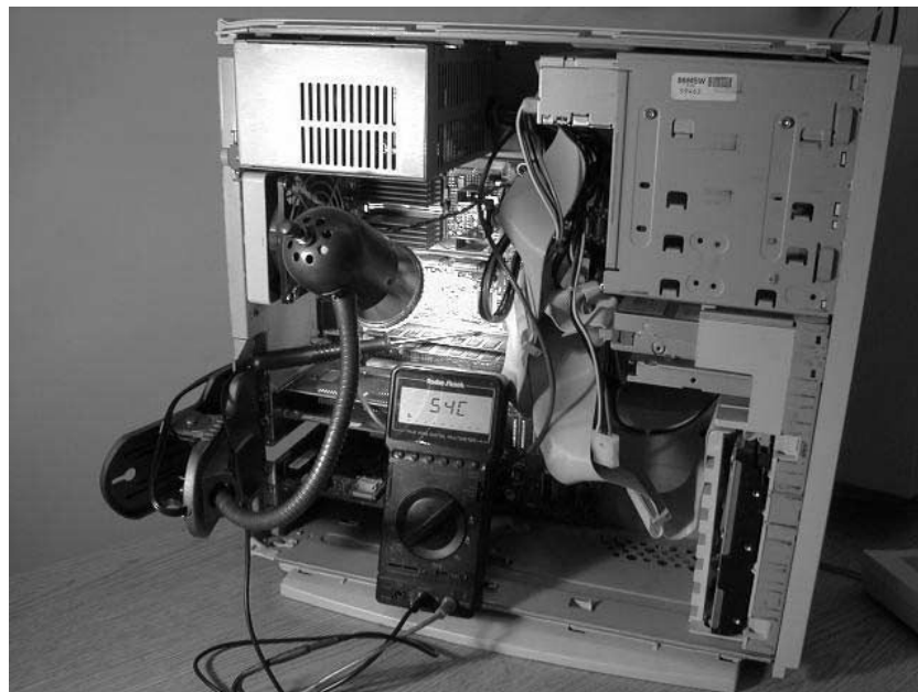
Figure 3.7: Experimental fault injection setup using the heat from a common light bulb [53]
