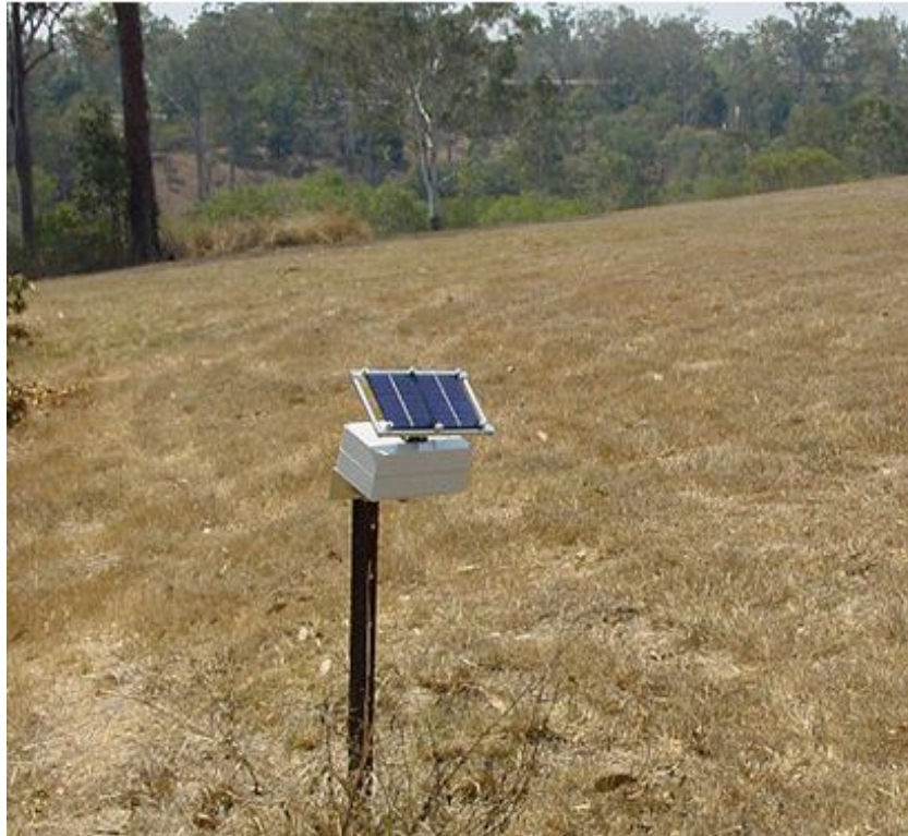
Figure 4.1: Remote sensor node of CSIROs Fleck sensor network, installed in a field [68]. Cropped to fit page.
