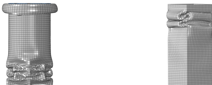
Figure 2.6: Post-test damage in circular (left) and squared (right) struts. Figures taken from p.441 in Paz Mendez et al. [20].
