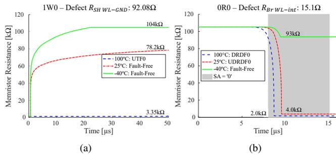
Fig. 5. Faults Detection: (a) 1w0; (b) 0r0.
