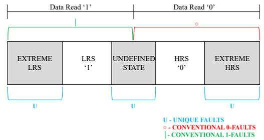
Fig. 1. Resistive states and faulty resistance intervals of ReRAM cells [14]. not ideal for the correct reading for the read circuit. So, this  $U$  state needs to be detected because it indicates misbehavior in the memristive device [8, 15]. According to the literature, four unique faults of ReRAMs are already described:
