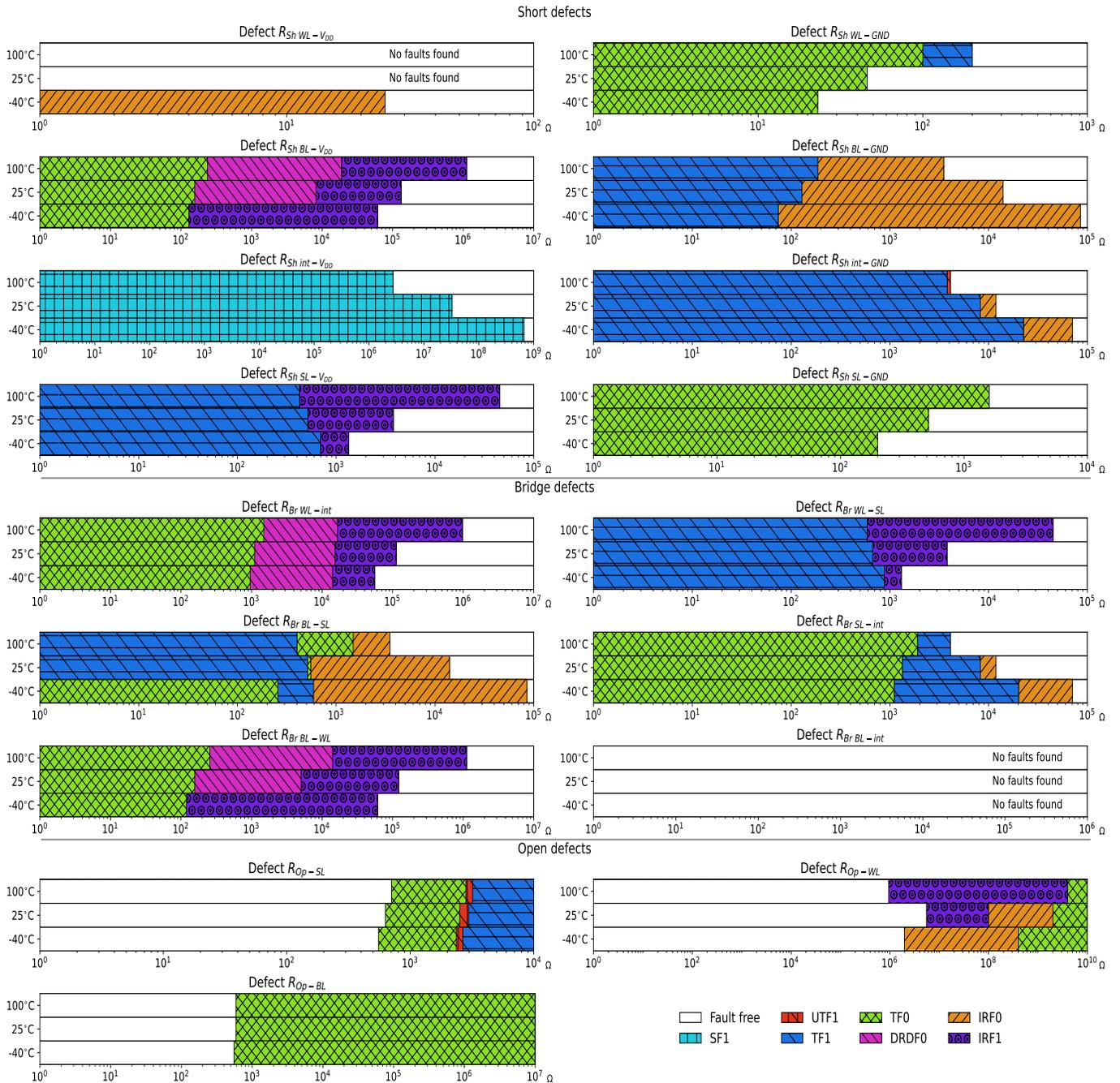
Fig. 4. Bar graphs of faults detected by resistive strength.
