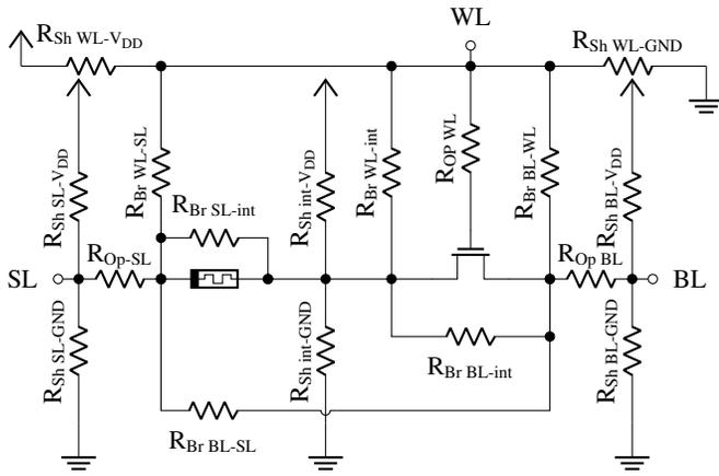
Fig. 2. Defect positions in a 1T1R cell.
