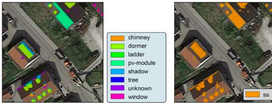
Figure 21: Roof superstructure detection into multi-class (left) and single-class (right); source: Prummer 2021
