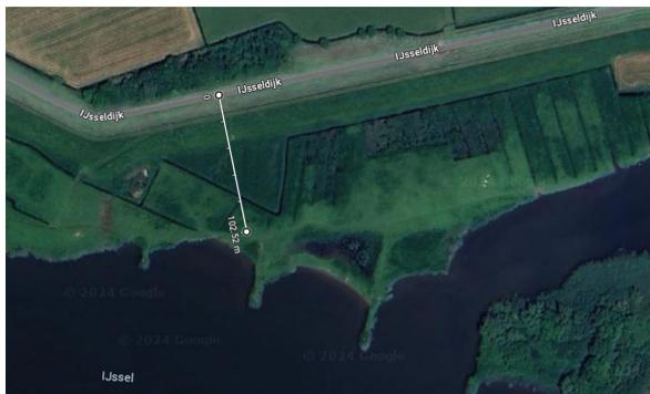
(a) Measurement of the foreshore length  $L_{foreshore}$ . The modelled foreshore lengths are normal to the dike trajectory, and the direction is shown in the figure by the white line.
