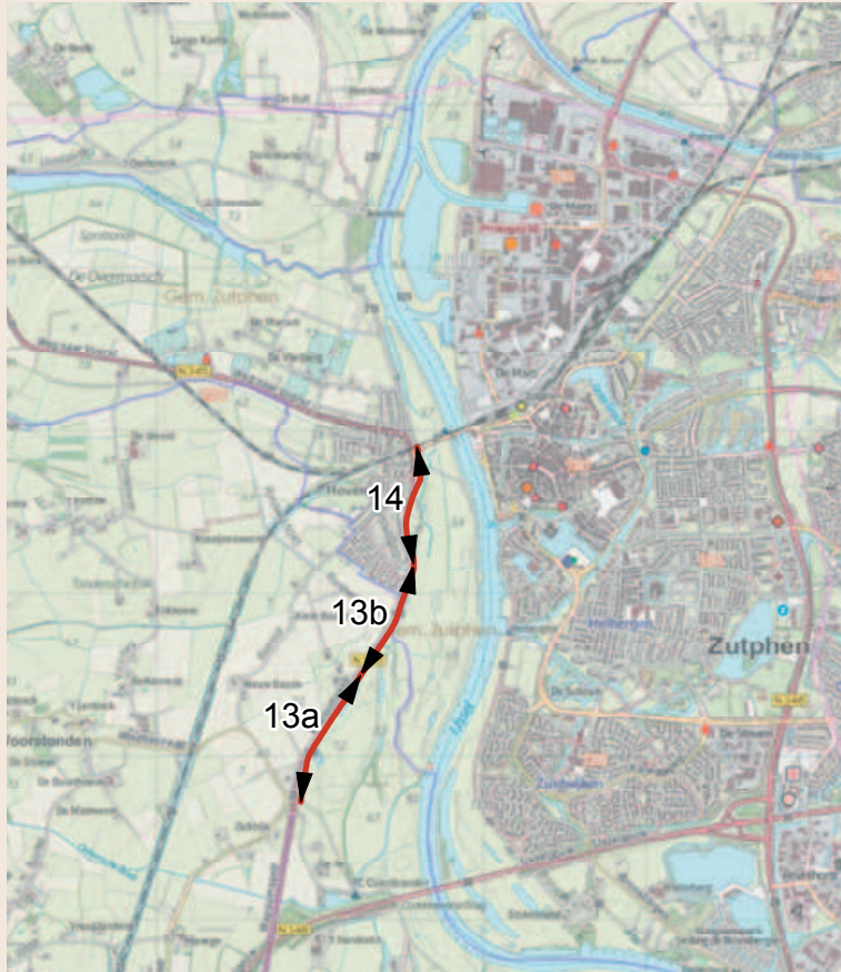
Figure 1. Levee system considered in the case study, three levee segments, 13a, 13b, and 14, which protect agricultural land and the western part of Zutphen from the IJssel River.
