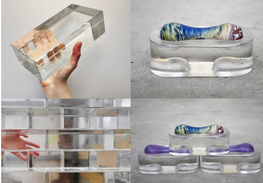
Figure 3: Left: Adhesively bonded unit and system; Right: interlocking unit and system
