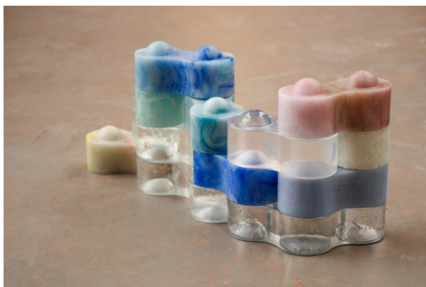
Figure 9: Prototype using E1 and E2 glass blocks from clear glass and recycled mouth-blown coloured glass
