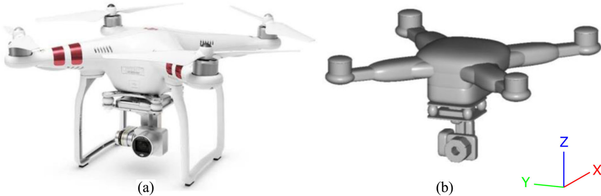
Figure 1. DJI Phantom III UAS used in impact modelling: (a) real-world system and (b) multibody system (MBS) model developed in MADYMO 11 . The two landing skids are neglected in the MBS model since they are such flexible that their impact effect is negligible [11].
