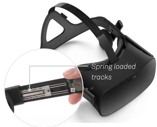
Figure 34 Automatic size adjustment
