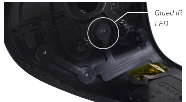
Figure 63 Glued IR LEDs
