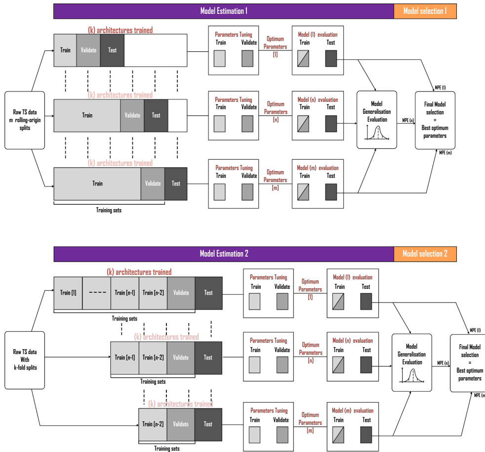
Fig. 6. Nested validation procedures – top: Nested Rolling-Origin Validation (NROV) – bottom: Nested Adjusted-k-fold Validation (NAK-foldV).
