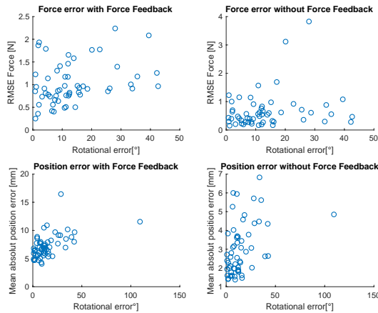
Fig. 8. The root mean square error and position error during the finding the hole phase are plotted against the rotational error of the stiffness ellipse in comparison with the ideal stiffness ellipse rotation. The first column depicts bilateral setting and the second column unilateral setting. The first row shows the root mean square error and the second row the position error.
