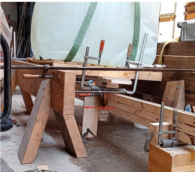
FIGURE 110: PHOTAGE OF WATER PLACING WATER TANK ON TOP OF THE BEAM (OWN WORK)
