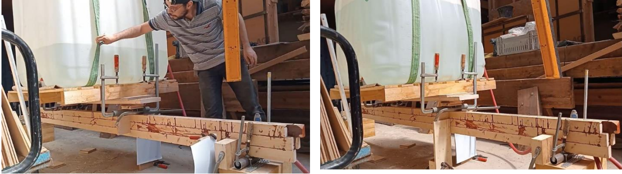
FIGURE 102: MEASURING THE LOAD FROM WATER LEVEL (OWN WORK)
