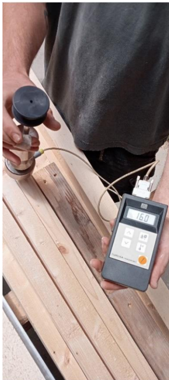
CHECKING THE MOISTURE CONTENT BEFORE LAMINATING
