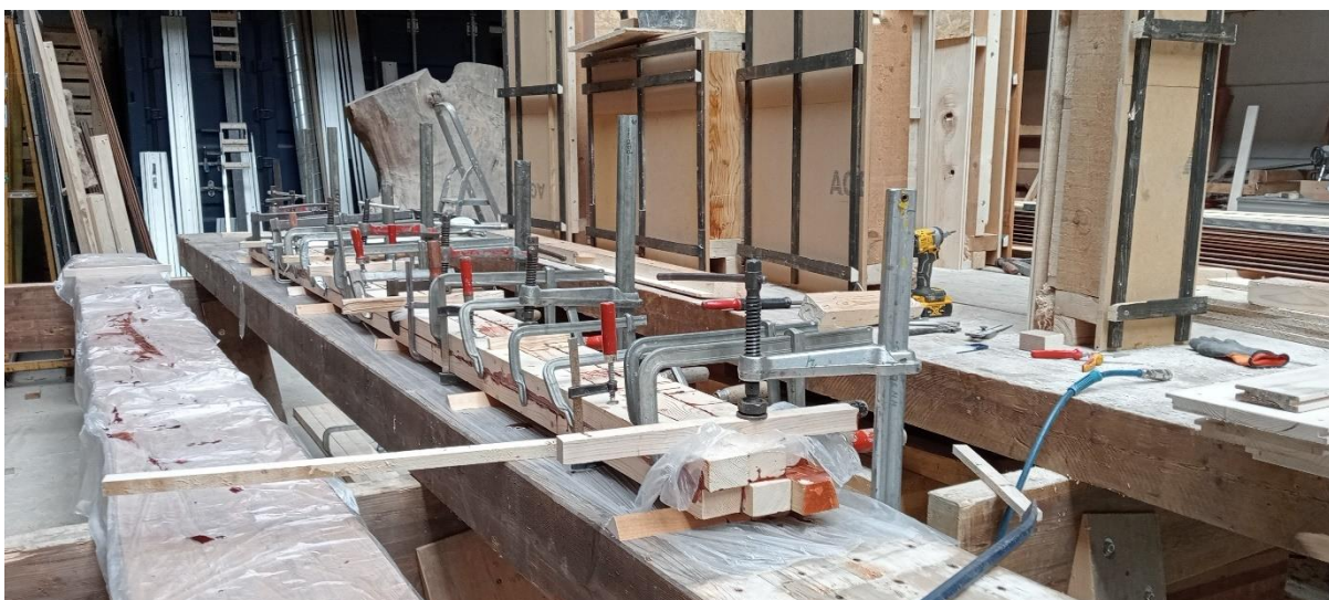
FIGURE 79:CLAMPING AFTER GLUEING (OWN WORK)
