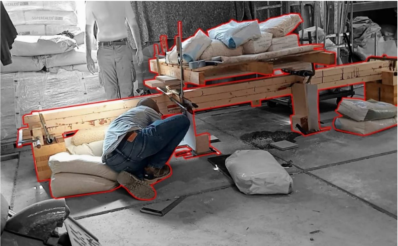
FIGURE 96: LOADING USING SANDBAG(OWN PHOTO)
