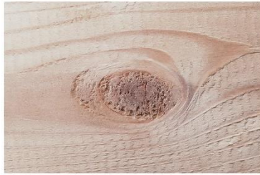
GRAIN INTERRUPTED BY BIG KNOTS (AVOIDED)
