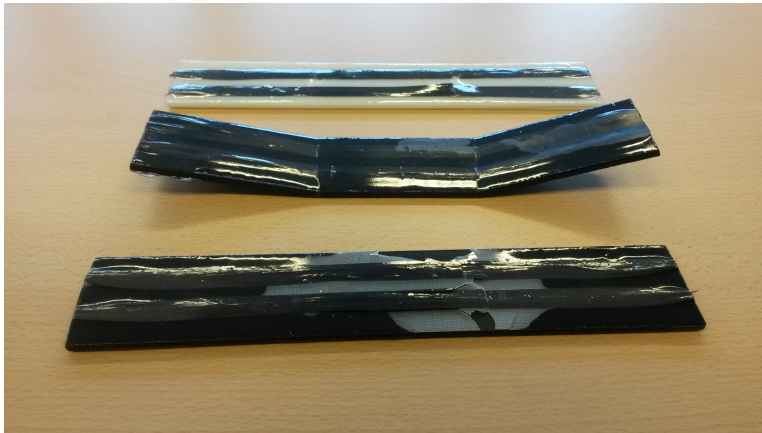
Figure 9.2: 3D printed samples post fracture. Top: ABS M30, Middle: PC-ABS, Bottom: Nylon.
