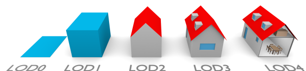
Figure 1. A building represented in LOD0 to LOD4 (image from Biljecki et al. (2016a)).
