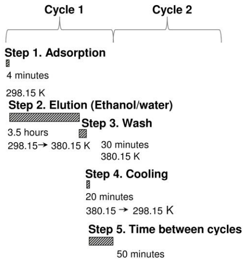
Figure 6.12. Cyclic operation for two batch cycles; Adsorption and recovery of ethyl acetate on column packed with Sepabeads SP20SS resin ( L=2m , D=0.08m )
