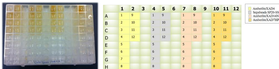
Figure 3.3 Schematic view of a 96-well plate filled with resin and samples
