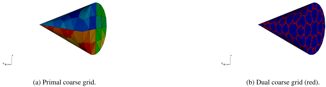
Fig. 6. The multiscale coarse grids used for the simulation in the cone-shaped domain.
