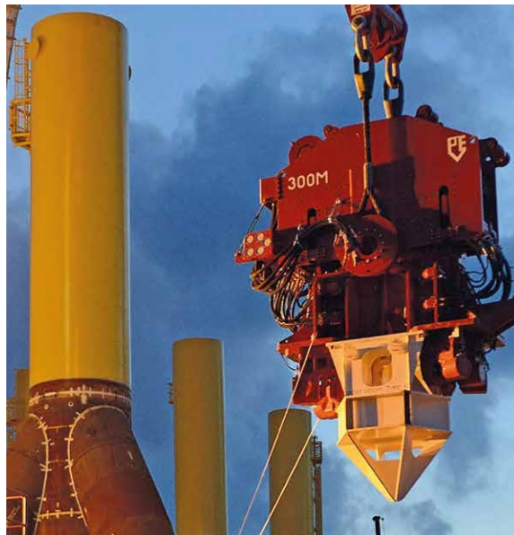
Figure 5.38: Dieseko's 300MU vibratory tool for the installation of piles for Tripod foundations [86]
