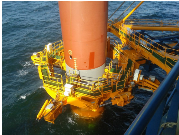
Figure 5.43: Pile gripper frame on Aelus vessel [94]
