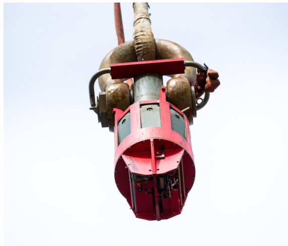
Figure 5.49: Combi lifting spread by IQIP [103]
