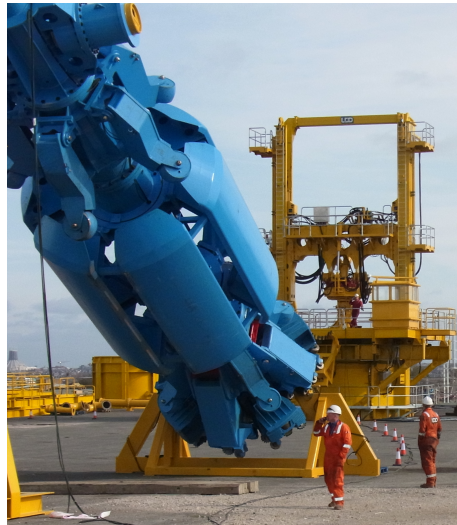
Figure 4.8: LD 5000 drill, for relief drilling foundation piles [39]
