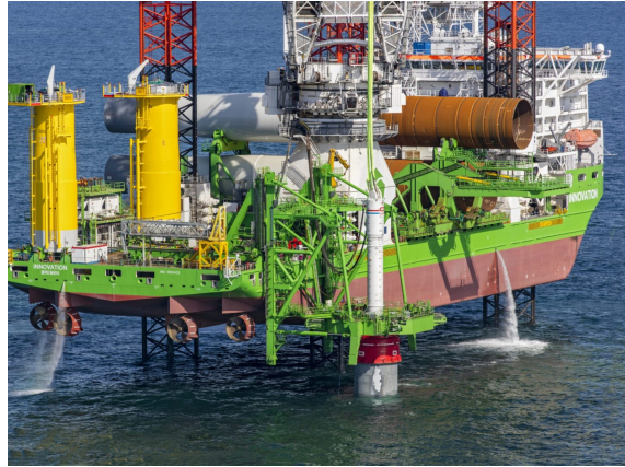
Figure 5.48: Pendulum design monopile gripper for the vessel Innovation [101]
