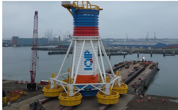
Figure 5.56: T-NMS-10000 noise mitigation system by IQIP [121]
