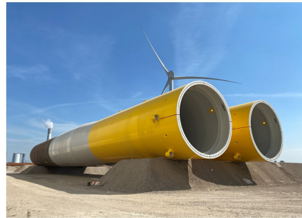
(b) TP-less monopile produced by Sif [21]
