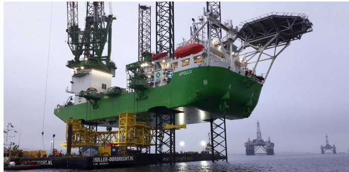
Figure 5.50: Under-deck hanging pre-piling template for the Apollo vessel by DEME [104]
