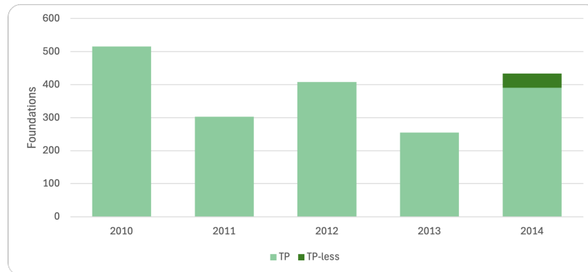
Figure 5.10: Transition piece type used between 2010 and 2015
