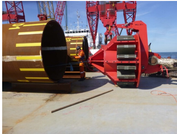
Figure 5.41: Internal lifting tool by IQIP [92]
