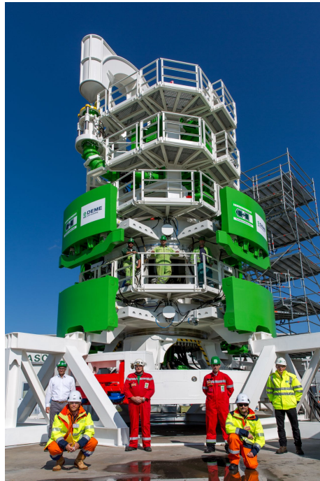
Figure 4.9: OFD 7700 offshore foundation drill by Herrenknecht [41]
