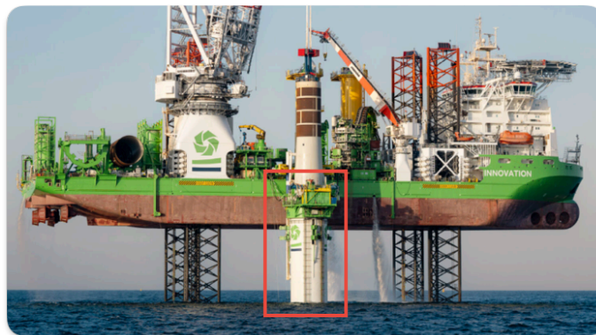
Figure 4.10: MODIGA monopile drilling and installation aid [44]
