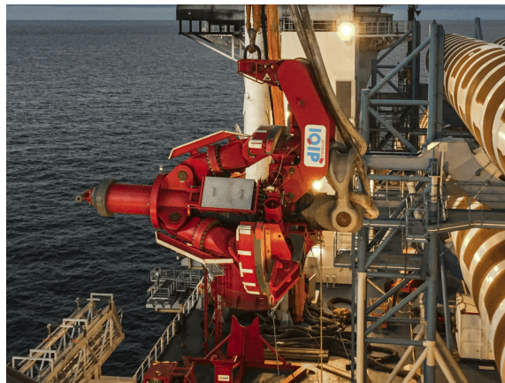
Figure 5.42: Flanged pile upending tool by IQIP [93]
