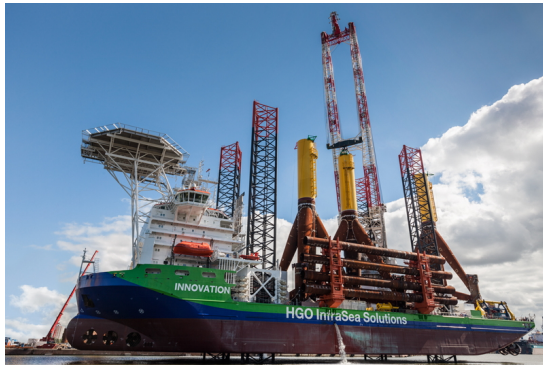
(b) Tripods loaded on deck of installation vessel Innovation, with their anchor piles, for Global Tech one wind farm [64]
