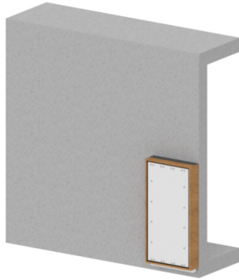
Step 9: The insulating panel is now hermetically sealed on all sides.
