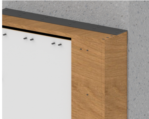
Step 10: Vertical wooden plates compose the external skin. Wood is fitted on the screw threads. A space is kept between the wooden plates to accommodate the movements due to thermal expansion.
