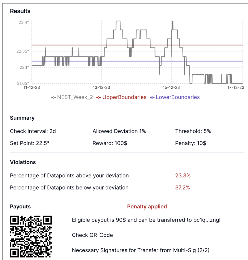
Figure 5: Evaluation of data in the application based on the contract terms and data set to calculate payouts. Authenticity of the data and contract can be checked against the timestamps. The invoice is created and needs to be signed by both the contractor and owner.
