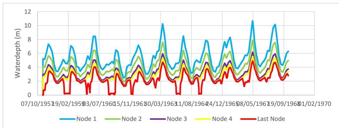
Figure B. 14.1 Water depth in Euphrates when the cross-section of branch 4 decreases 20%
