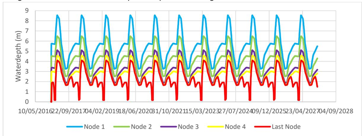
Figure B. 4.1 Water depth in Euphrates when all nodes are open and Branch 1 is closed
