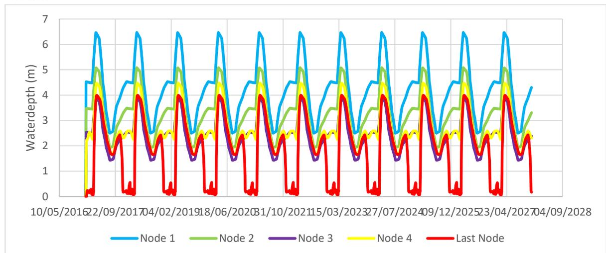
Figure B. 6.1 Water depth in Euphrates when all nodes are open and branch 5 is closed
