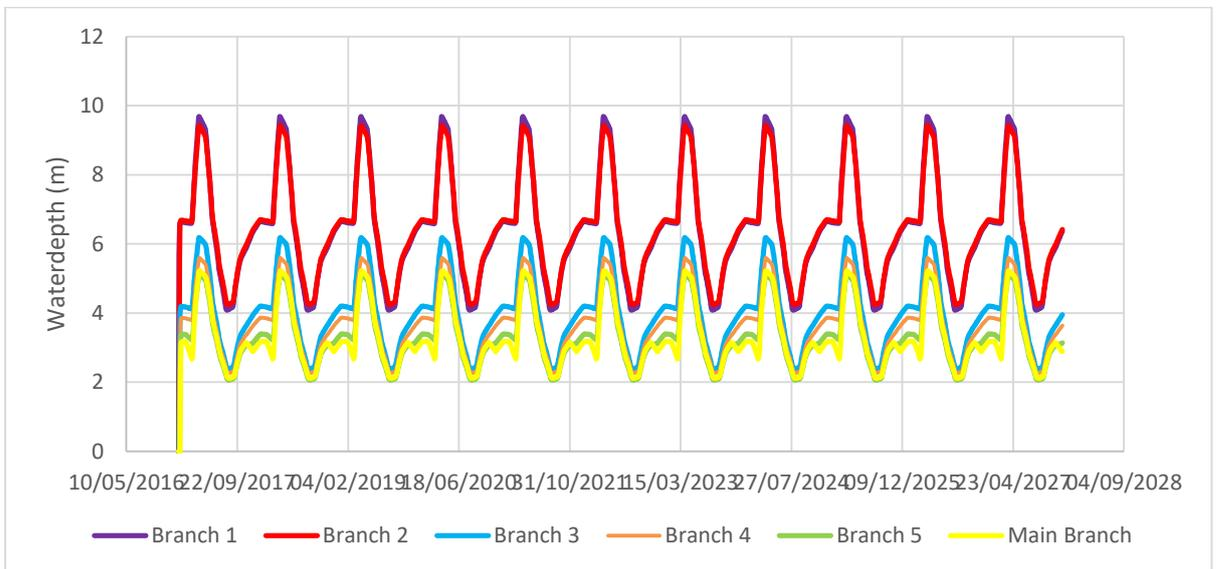
Figure B. 5.2 Water depth in Euphrates branches when all nodes are open and branch 1 and 2 are closed
