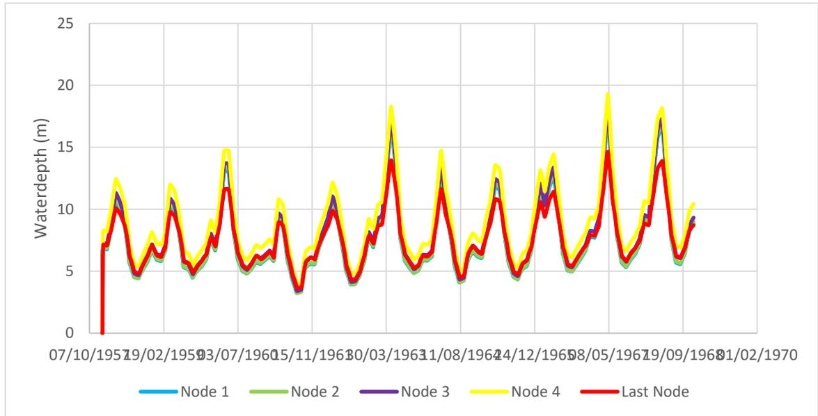
Figure B. 16.1 Water depth in Euphrates when there are no branches
