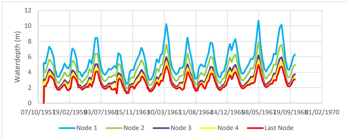
Figure B. 9.3 Water depth in Euphrates when the last 2 irrigation Nodes are open
