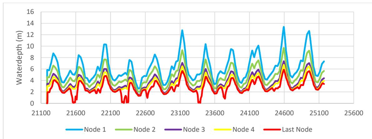
Figure B. 11.2 Waterdepth in Euphrates when the cross-section of branch 1 decreases 80%
