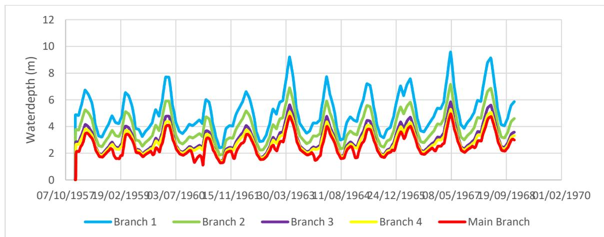
Figure B. 10.2 Water depth in Euphrates branches when the first 16 irrigation nodes are open
