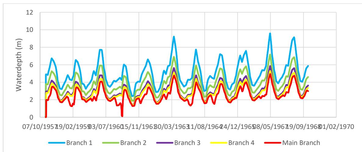
Figure B. 9.2 Water depth in Euphrates branches when the last 3 irrigation Nodes are open
