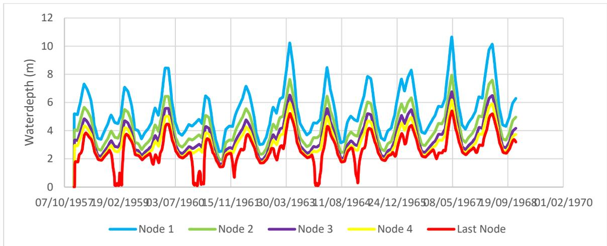
Figure B. 14.3 Water depth in Euphrates when the cross-section of branch 4 is closed
