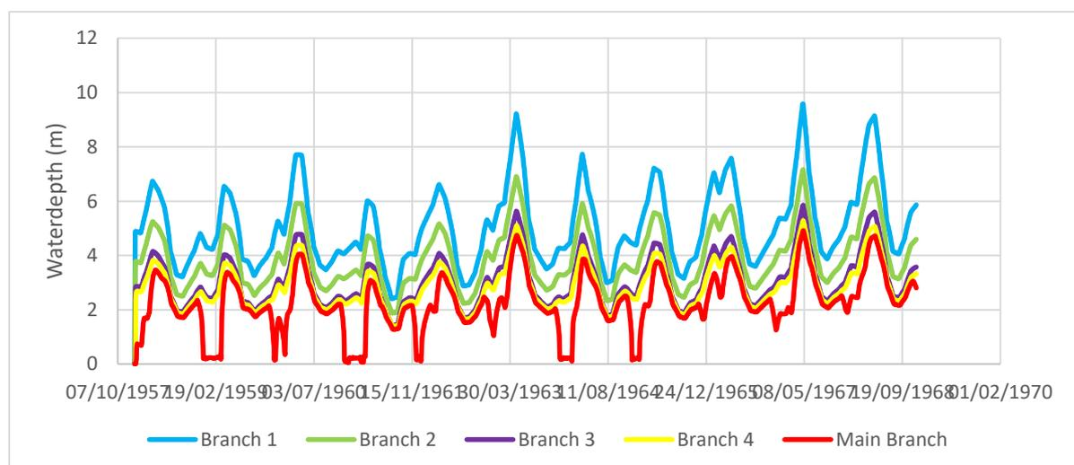
Figure B. 8.2 Water depth in Euphrates branches when all nodes are open
