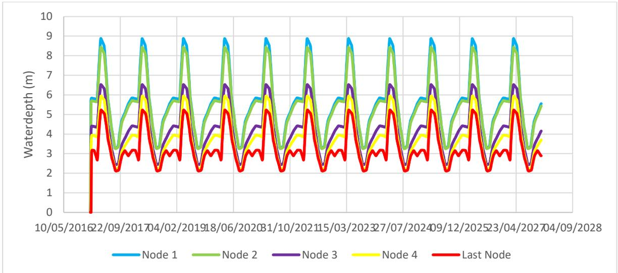
Figure B. 5.1 Water depth in Euphrates when all nodes are open and branch 1 and 2 are closed
