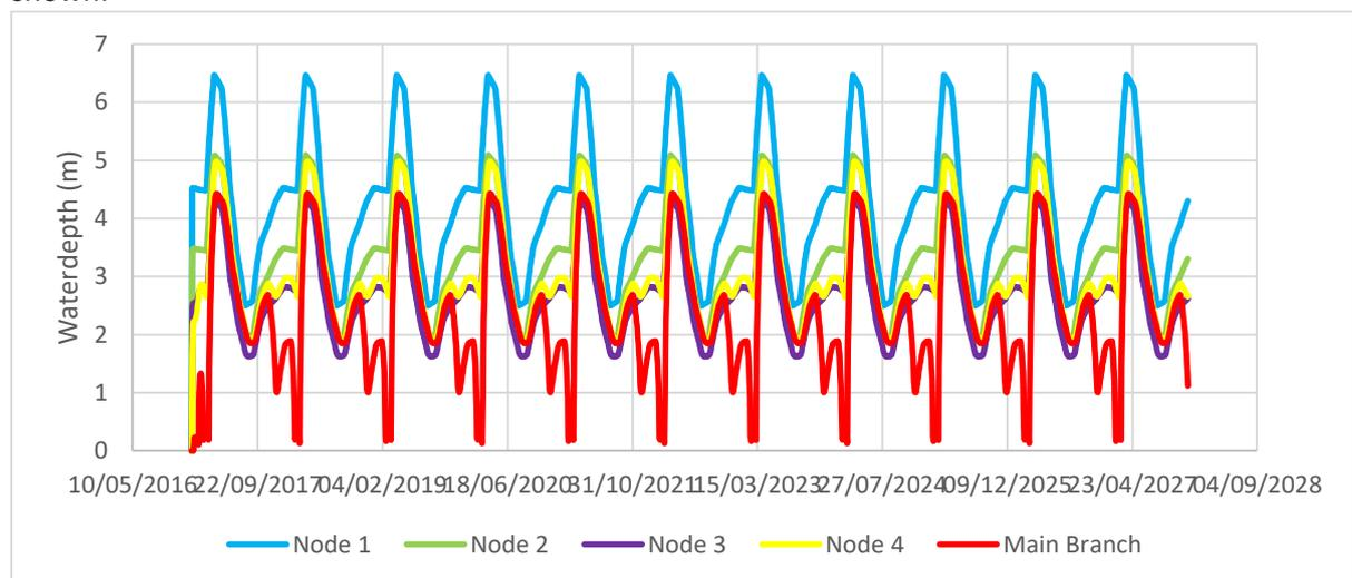
Figure B. 7.1 Water depth in Euphrates when all nodes are open and branch 5 and branch 6 are closed
