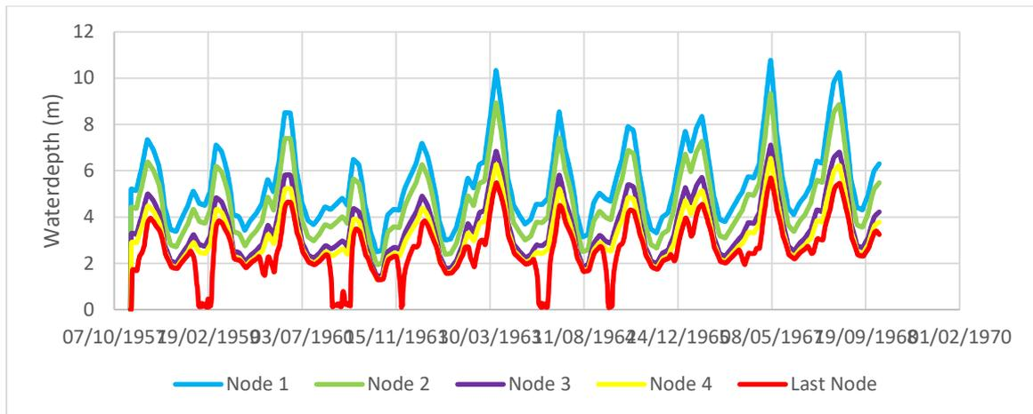
Figure B. 12.2 Discharge of Euphrates when the cross-section of branch 2 decreases 80%
