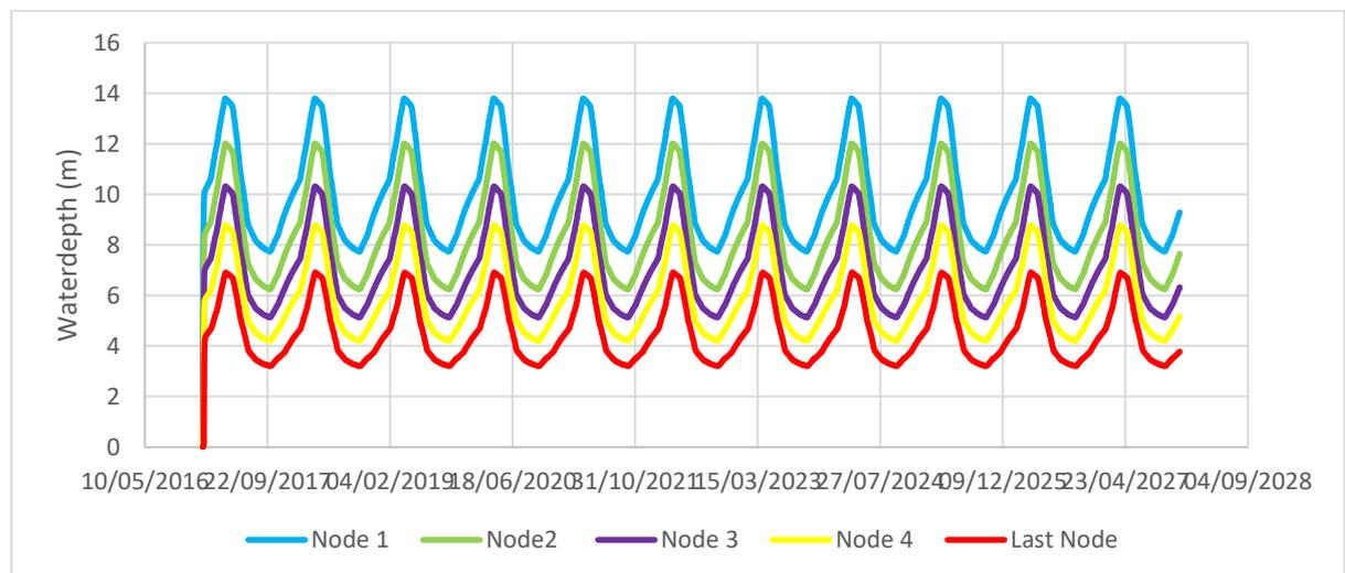
Figure B. 2.2 Water depth in Tigris when all nodes are open and with average flow
