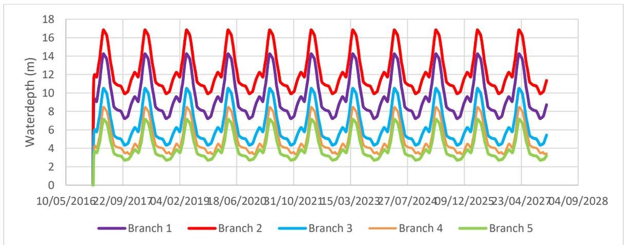
Figure B. 4.4 Water depth in Tigris branches when all nodes are open and Branch 1 is closed
