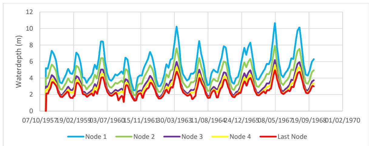
Figure B. 10.1 Water depth in Euphrates when the first 16 irrigation nodes are open
