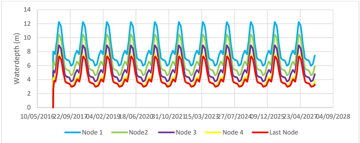
Figure B. 6.3 Water depth in Euphrates when all nodes are open and branch 5 closed
