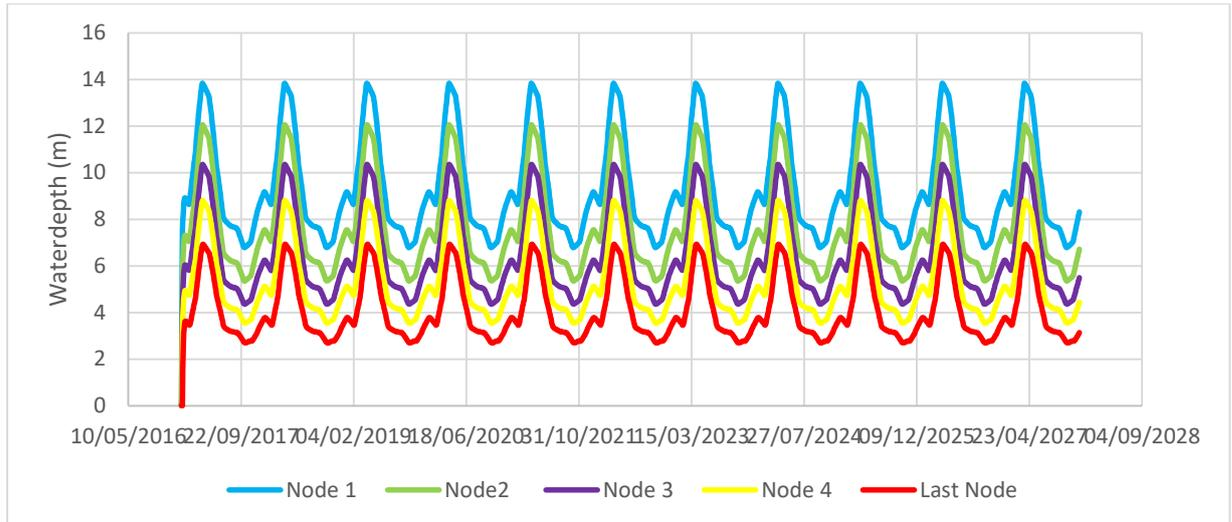
Figure B. 4.3 Water depth in Tigris when all nodes are open and Branch 1 is closed
