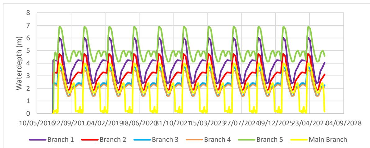
Figure B. 6.2 Water depth in Euphrates branches when all nodes are open and branch5 is closed
