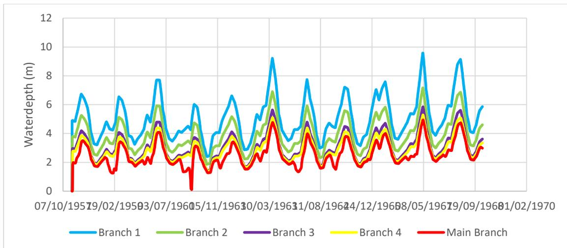
Figure B. 9.4 Water depth in Euphrates branches when the last 2 irrigation nodes are open
