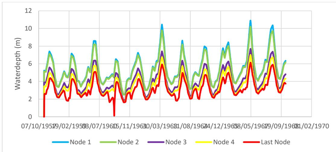
Figure B. 11.3 Water depth in Euphrates when the cross-section of branch 1 is closed
