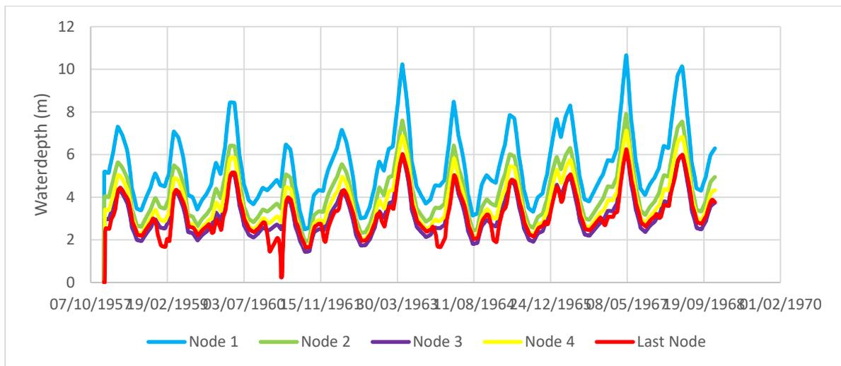
Figure B. 14.6 Water depth in Euphrates when the cross-section of branch 5 is closed
