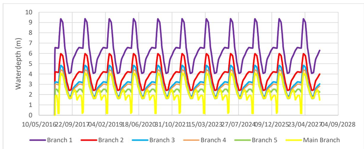
Figure B. 4.2 Water depth in Euphrates branches when all nodes are open and Branch 1 is closed
