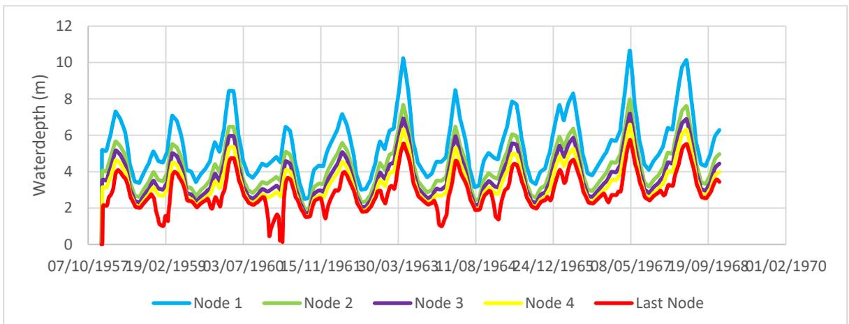
Figure B. 13.3 Water depth in Euphrates when the cross-section of branch 3 is closed
