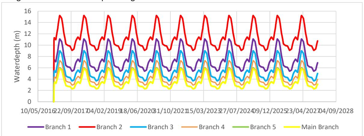
Figure B. 1.4 Water depth in Tigris branches when there are no nodes and with minimum flow
