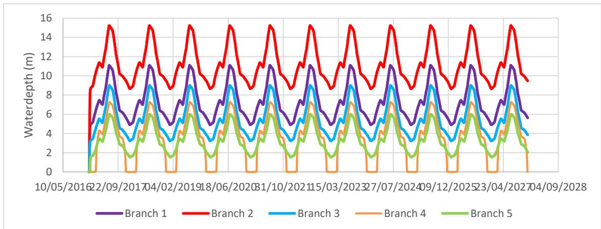
Figure B. 3.4 Water depth in Euphrates branches when all nodes are open and with minimum flow
