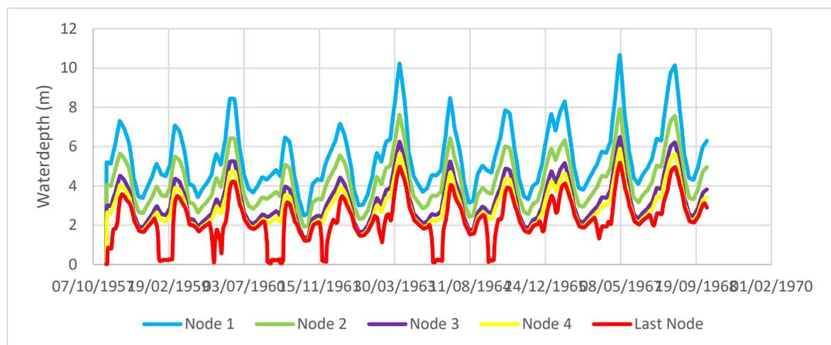
Figure B. 14.2 Waterdepth in Euphrates when the cross-section of branch 4 decreases 80%
