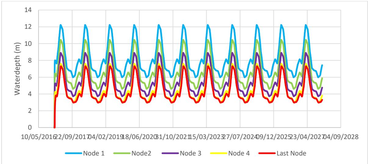
Figure B. 7.3 Water depth in Tigris when all nodes are open and branch 5 and branch 6 are closed
