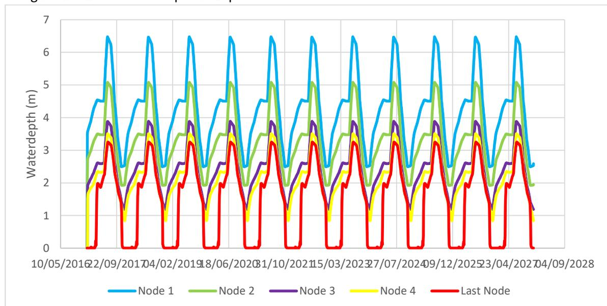
Figure B. 3.1 Water depth in Euphrates when all nodes are open and with minimum flow
