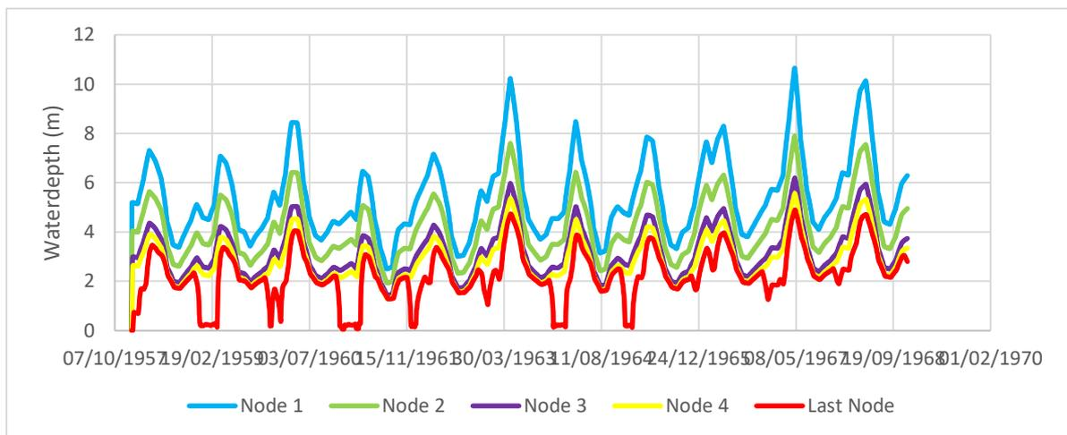
Figure B. 14.4 Water depth in Euphrates when the cross-section of branch 5 decreases 20%
