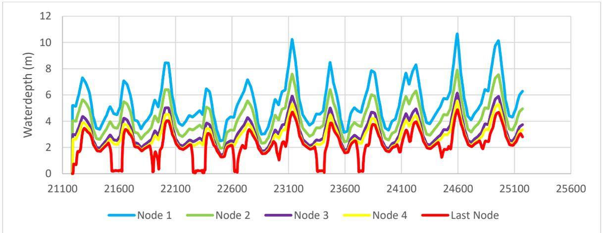
Figure B. 13.1 Water depth in Euphrates when the cross-section of branch 3 decreases 20%
