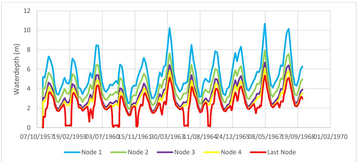
Figure B. 13.2 Waterdepth in Euphrates when the cross-section of branch 3 decreases 80%
