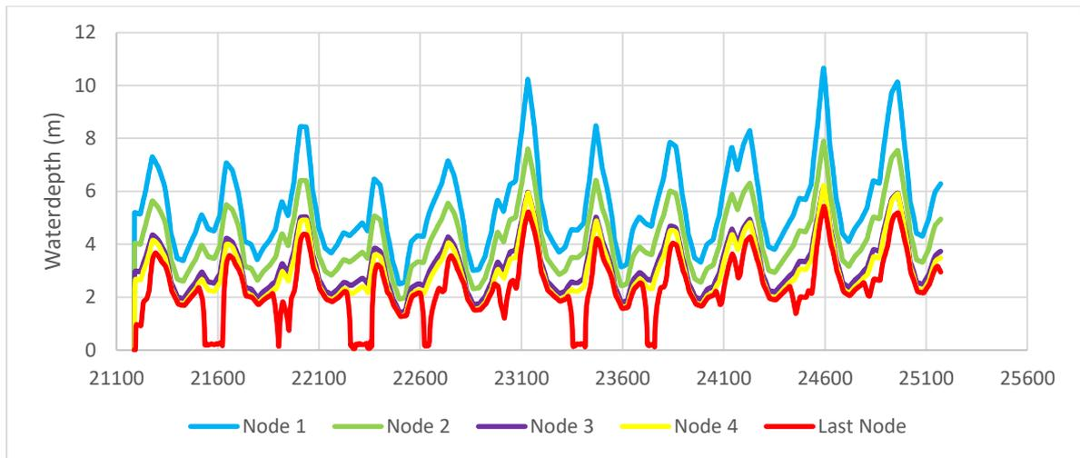
Figure B. 14.5 Waterdepth in Euphrates when the cross-section of branch 5 decreases 80%
