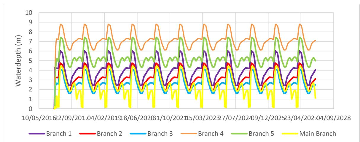
Figure B. 7.2 Water depth in Euphrates branches when all nodes are open and branch 5 and branch 6 are closed
