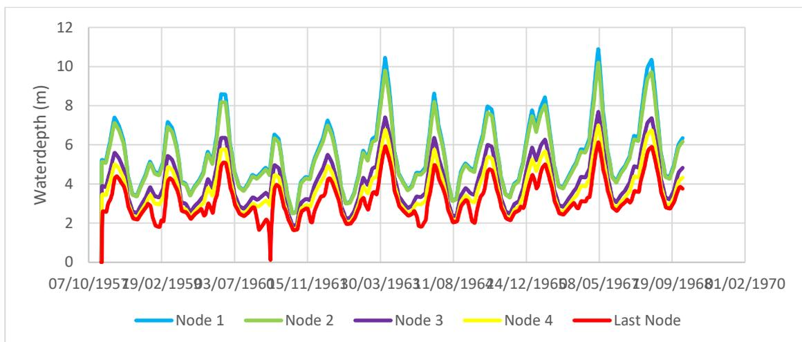
Figure B. 12.3 Water depth in Euphrates when the cross-section of branch 2 is closed
