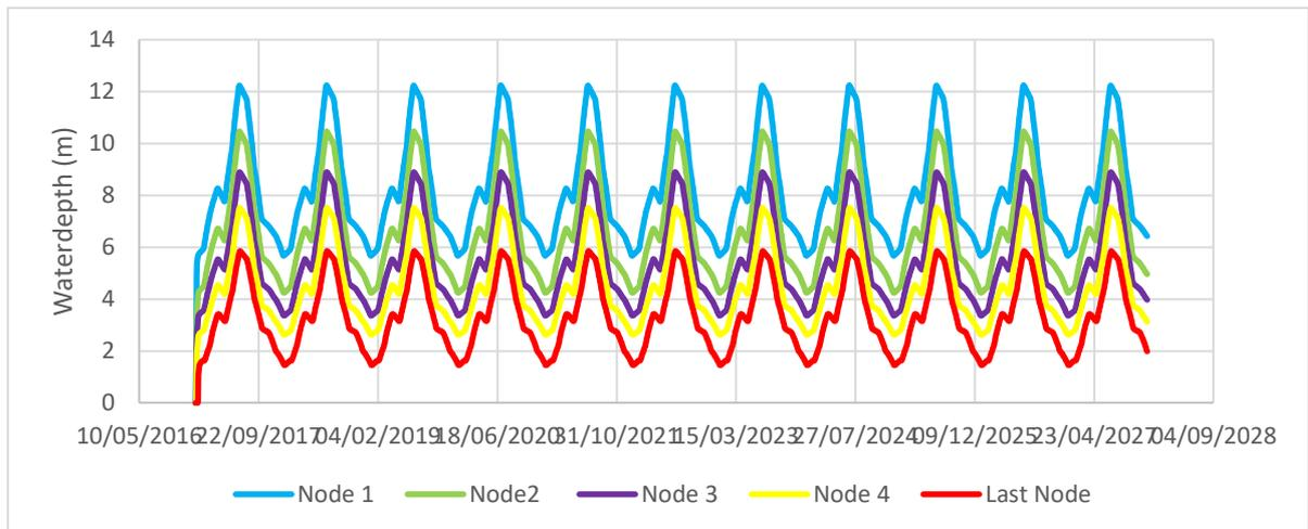
Figure B. 3.3 Water depth in Tigris when all nodes are open and with minimum flow
