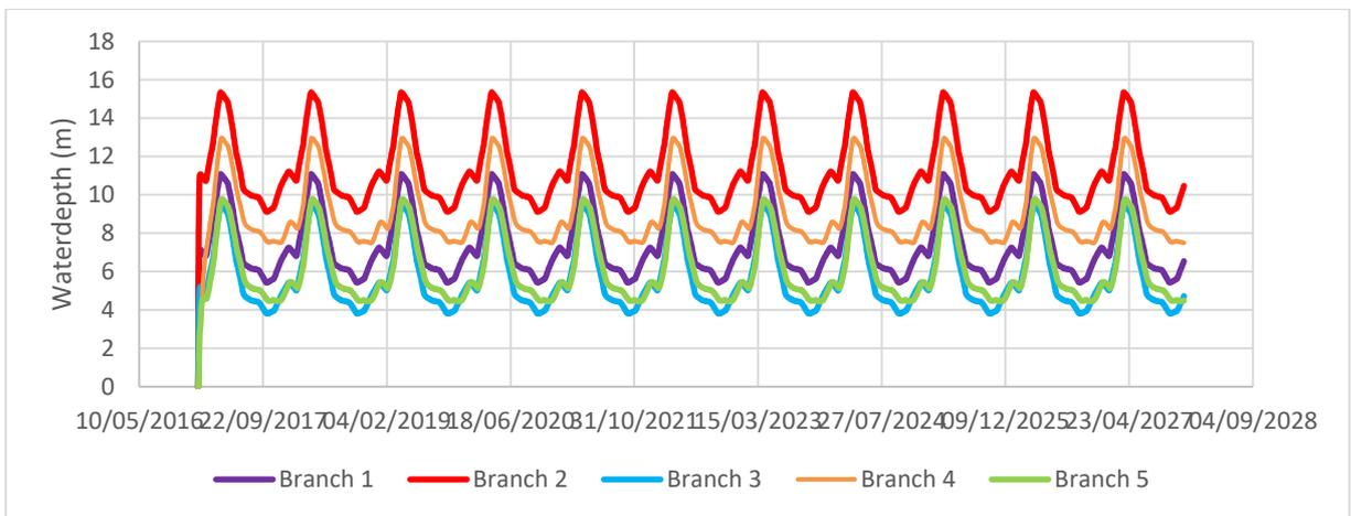
Figure B. 7.4 Water depth in Tigris branches when all nodes are open and branch 5 and branch 6 are closed
