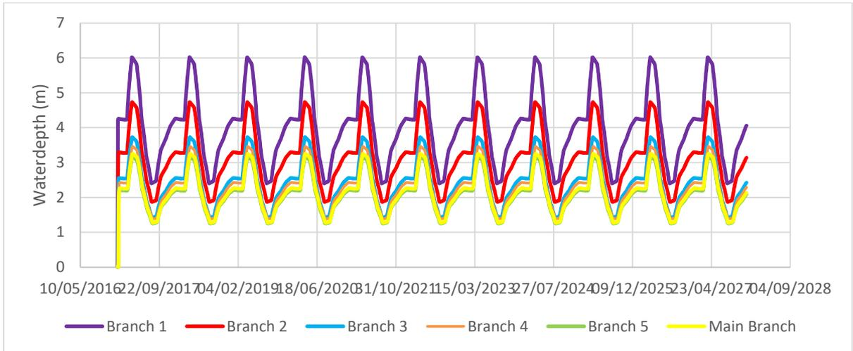
Figure B. 1.2 Water depth in Euphrates branches when there are no nodes and with minimum flow
