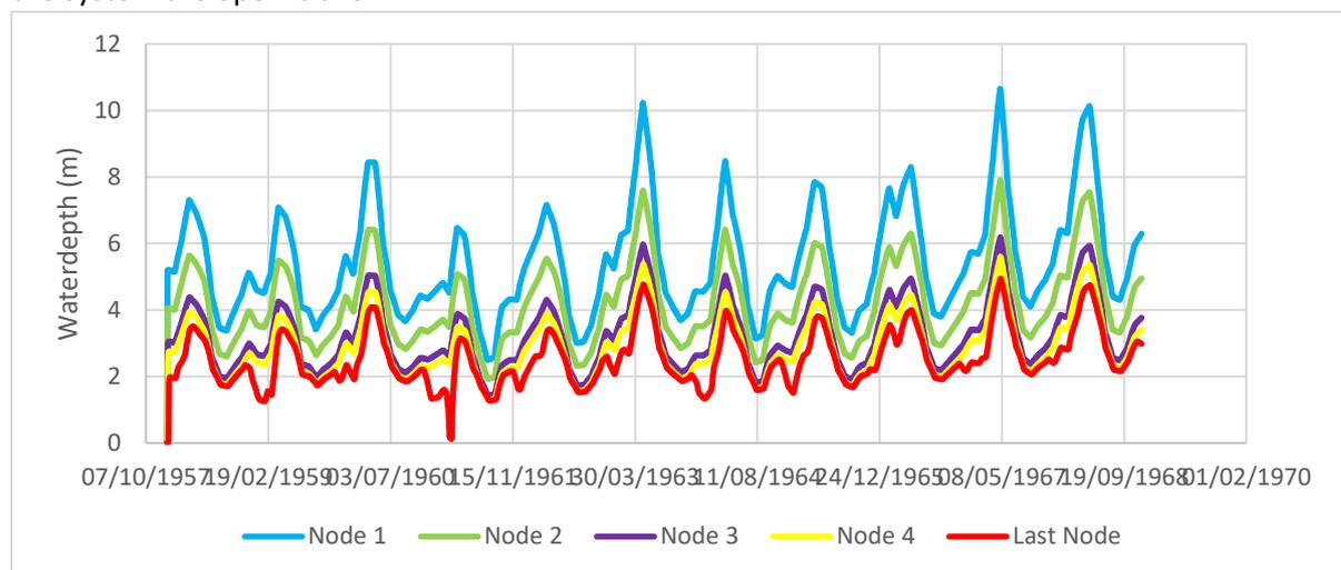
Figure B. 9.1 Water depth in Euphrates when the last 3 irrigation Nodes are open
