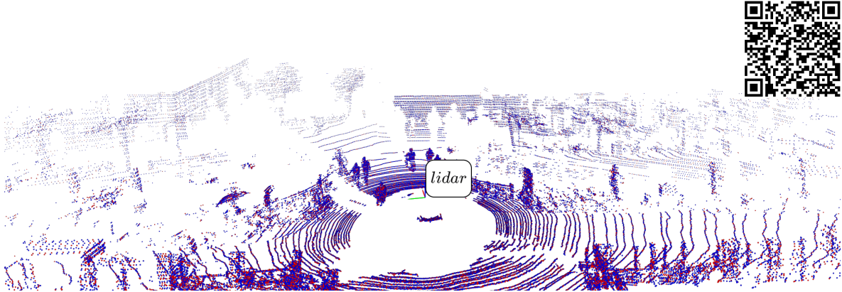
Figure 4-3: Original(red) and reconstructed using TMC3(blue) LiDAR data. PSNR-NN: 106.69. BPP: 23.47. Scan QR Code or click on link for 3D Render.
