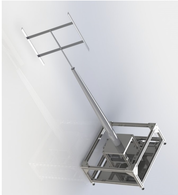
Figure 3.1: Force balance with VAWT setup
