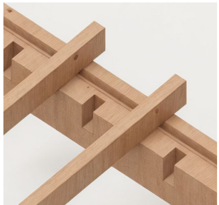
INT BEAM - EXT BEAM JUNCTION
