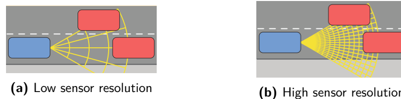
Figure 2-1: Schematic example of low and high sensor resolution with respect to object size in automotive tracking applications. Borrowed from Granström et.al. (2014) [1].
