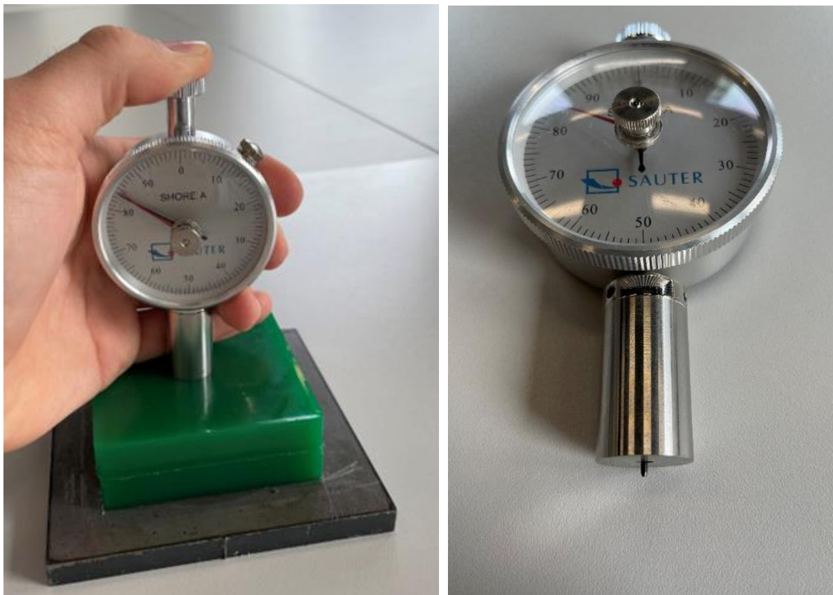
Figure 3.2. Shore hardness measurement of a polyurethane (pictures made on 19-4-2022)
