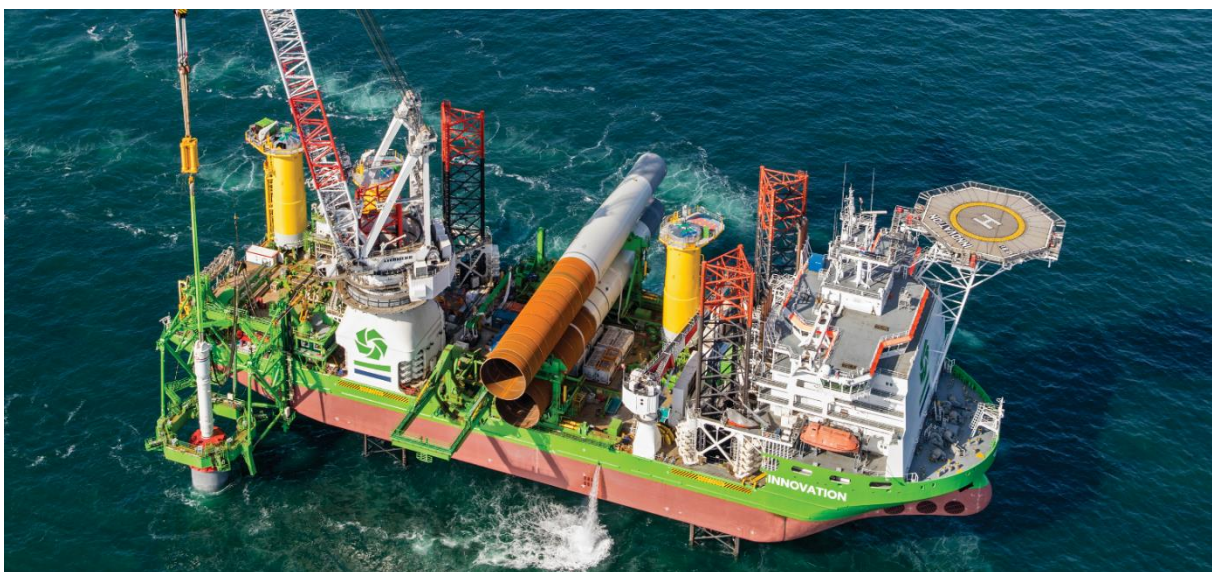
Figure 1.3. Friction-based monopile sea fastening (DEME, 2018)
