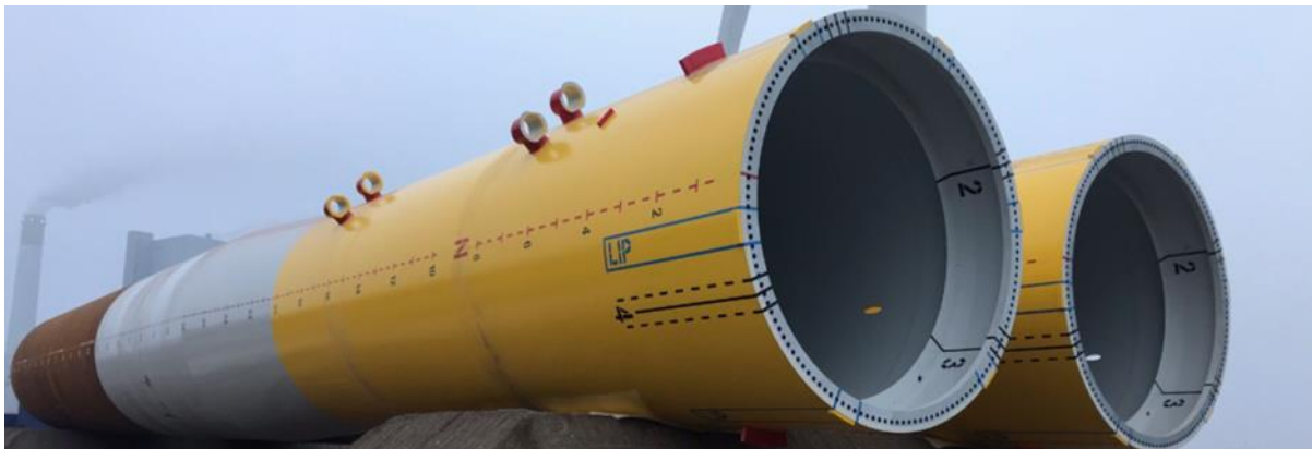
Figure 3.17. Coated monopile (Sif Group, 2021)
