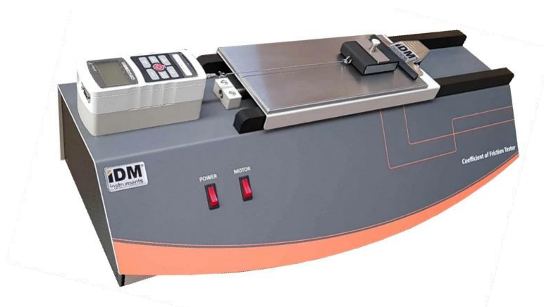
Figure 4.6. Horizontal plane friction measurement device (IDM instruments, n.d.)
