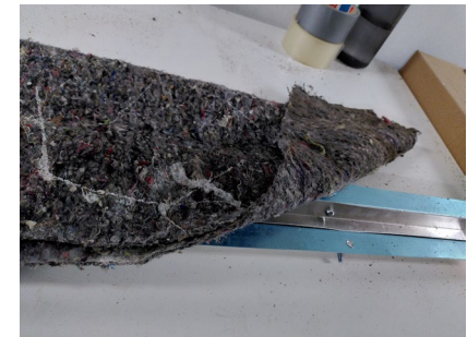
Lay the mat over the profile and push it in the profile's slot
