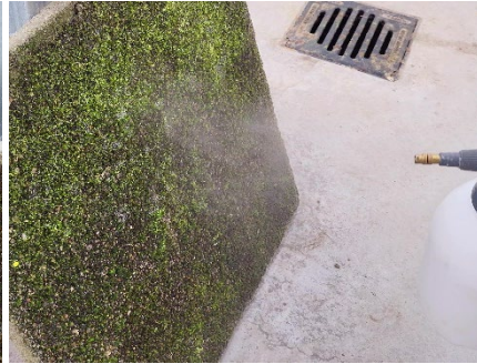
Figure 18: test set-up B, water through the air using a spray nozzle.
