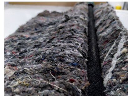
Lay the soaker hose in the slot
