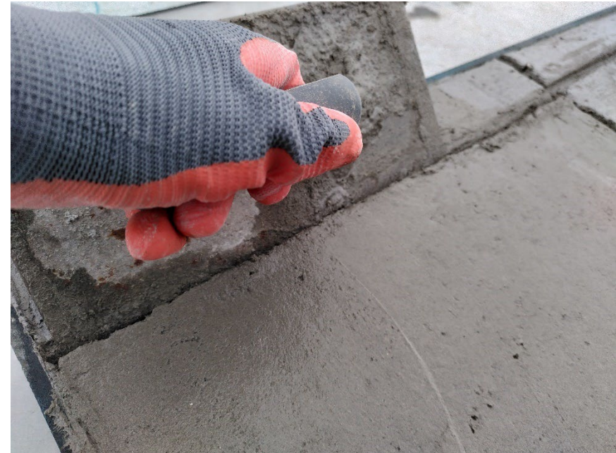
Figure 21: Concrete panels in their mould. Some prototypes include carving indents in the concrete.
