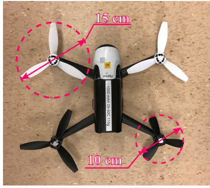
Fig. 12. A Bebop 2 quadrotor with one damaged rotor.
