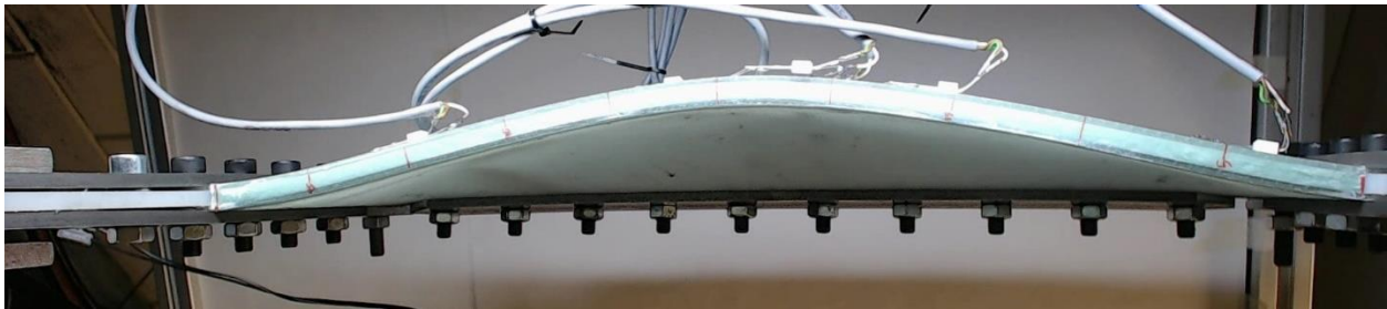
Figure 7.19 - Testing of TEB03b with a redesigned full-steel posterior clamp.
