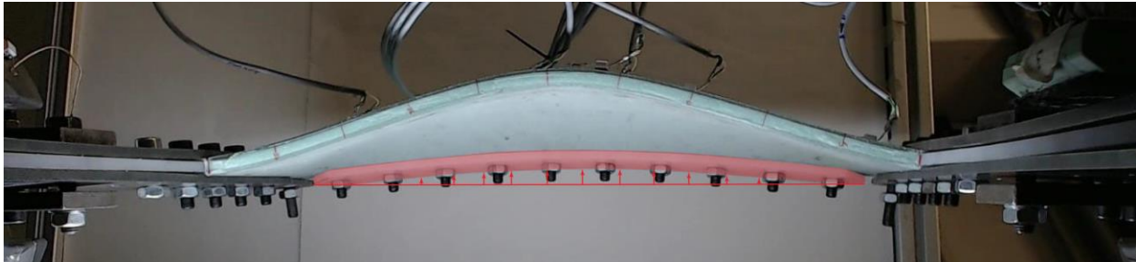
Figure 7.17 - Posterior clamp buckling due to insufficient stiffness of nylon pieces.
