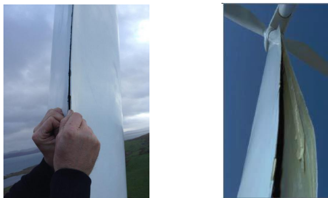
Figure 1.3 a) Trailing edge debonding of operational wind turbine blade. b) Catastrophic failure of blade induced by trailing edge debonding. Obtained from [5]
