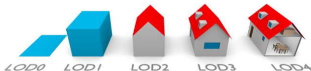
Figure 1. The levels of detail for buildings in CityGML (Biljecki et al., 2016)
