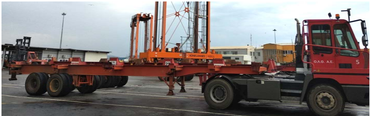
Figure 7 - Tractor - Trailer set for the horizontal transport of containers
