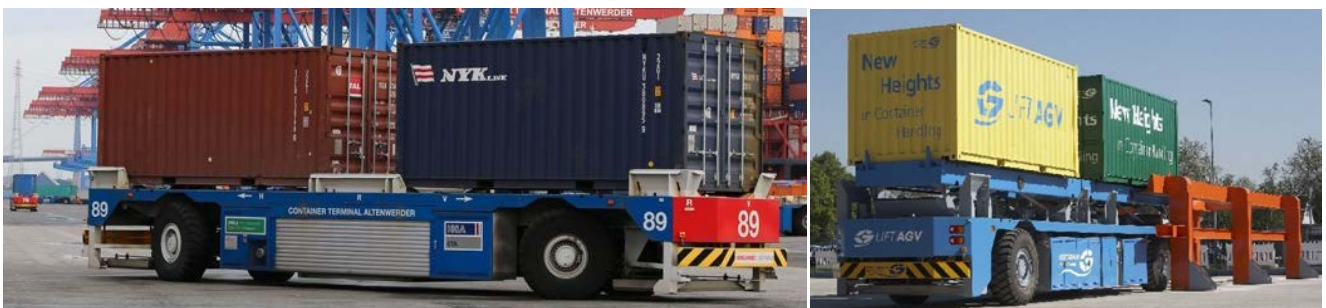
Figure 8 - Automatic Guided Vehicle (AGV) to the left [23] and lift - AGV to the right picture [24]
