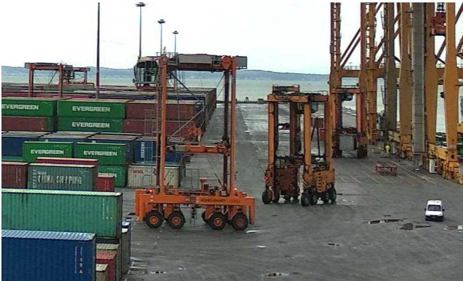
Figure 6 - 1 over 3 and 1 over 2 straddle carriers operating together for horizontal transport and for stacking of containers
