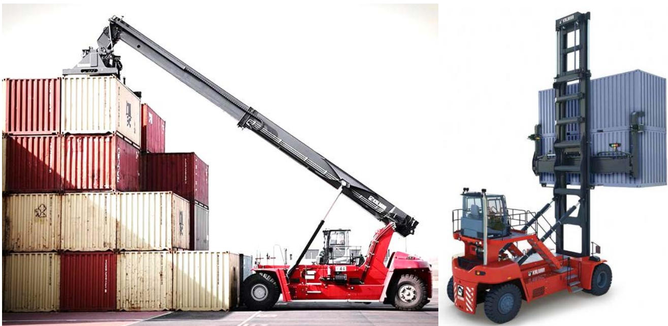
Figure 5 - Reach Stacker to the left and Front Lift equipment to the right picture [22]
