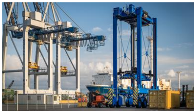
Figure 10 – The new 1 over 3 automated straddle carrier at the port of Auckland [18]
