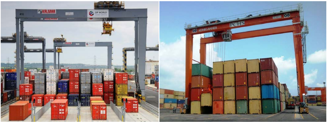
Figure 4 - Rail Mounted Gantry crane (RMG) to the left [21] and Rubber Tyred Gantry crane (RTG) to the right picture [20]
