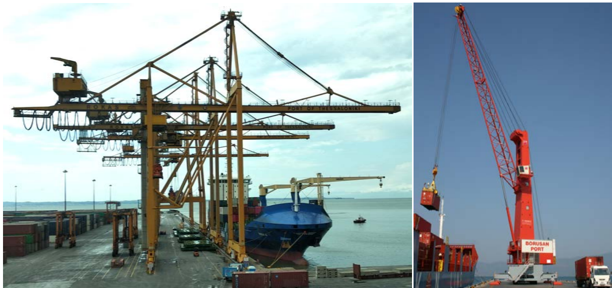
Figure 3 - Ship To Shore gantry crane to the left and Mobile Harbor Crane to the right picture [19]
