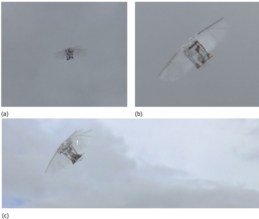
Figure 4.14: Quad-thopter In-flight Outdoor in various phases of the flight. (a) hover (b) semi-transitioned (c) fast forward flight.
