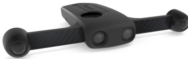
Figure 6.17: Parrot SLAMdunk vision system with a dual fish-eye lens at a baseline of 20 cm and an Nvidia Tegra TK1 processor.
