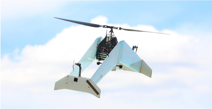
Figure 6.1: Novel hybrid UAV which combines a cyclic and collective pitch controlled main rotor with a biplane delta-wing and torque compensating tip rotors. The biplane concept adds structural rigidity and minimizes the lateral surface area to reduce the perturbations from turbulence during hover. The large main rotor allows efficient hovering flight while the cyclic control provides large control authority in hover.
