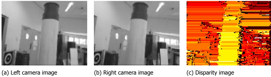
Figure 2.11: Sample disparity image if the 4g stereo vision system on 128 \times 96 pixels processed on a 168 MHz 32-bit DSP with a single camera port and only 196 kb of memory. In areas of low contrast, the algorithm propagates the disparity of the closest edge. While the disparity image is not state-of-the-art in terms of accuracy, in terms of memory and computational power, it nevertheless enables the 20 g robot to safely navigate.
