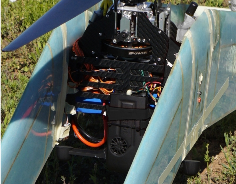
Figure 6.18: The SLAMdunk vision system was mounted on the side of the center fuselage DelftaCopter looking away from the main rotor. In hovering flight, this means the camera has a perfect view of the ground, and in forward flight, the camera looks backward. Thanks to the wide field of view fisheye lenses the camera can also look vertically down during forward flight.
