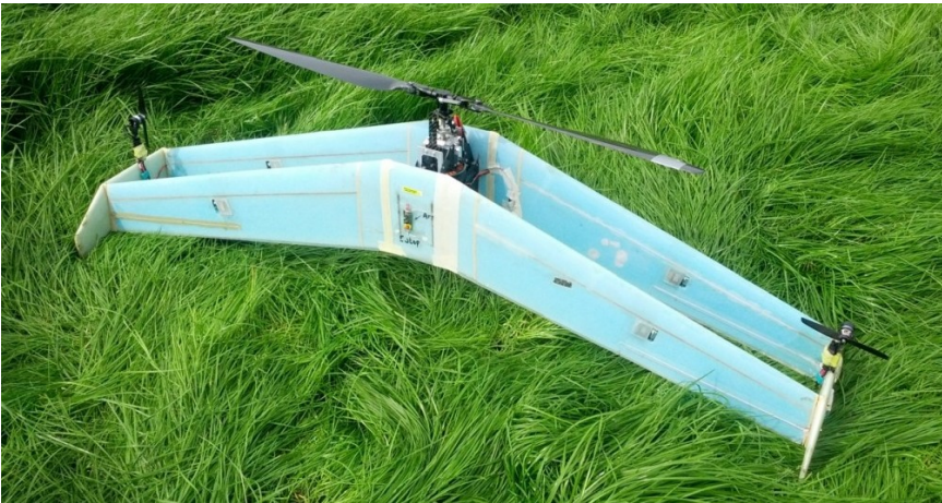
Figure 5.1: Novel hybrid Unmanned Air Vehicle featuring a cyclic and collective pitch controlled rotor combined with a biplane deltawing.
