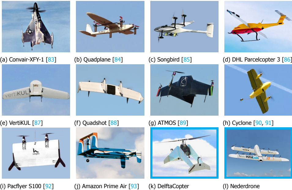
Figure 1.3: Hybrid aircraft and UAVs that can take-off and land vertically while using fixed wings to increase flight efficiency during fast forward flight. Robots in the blue boxes are proposed in this research.
