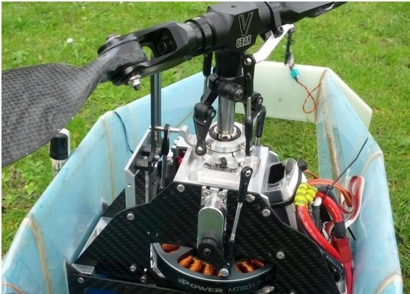
Figure 6.16: Close up of the rotor head of the DelftaCopter. The swashplate has three leverage points at 120^\circ from each other. The collective pitch can reach from -40^\circ to 40^\circ , which is double that of a conventional helicopter. The blades have high camber, a high lift coefficient, and 25^\circ of blade twist from root to tip. Hovering flight is performed at a designed tip angle of attack of around 10^\circ with 1500 rpm. In forward flight, the tip angle of attack can change up to 50^\circ at 500 rpm. The root angle of attack is then about 75^\circ . Having blade twist is possible because the flow is always axial as the DelftaCopter transitions. This allows the rotor to be efficient from hover to fast forward flight.
