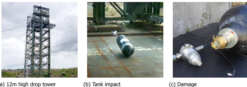
Figure 8.6: Drop-test of a hydrogen-filled cylinder on steel-covered concrete did cause a leak at the regulator but did not visibly damage the cylinder and did not lead to fire nor detonation.
