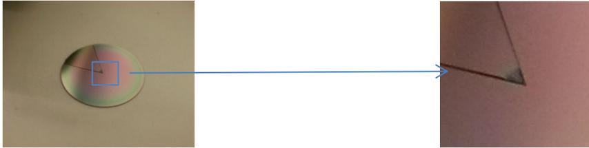
Figure 5.9: Image of the circular Al metal plate in the PECVD machine (left) after deposition of Glass, in the centre the chip is visible (right). In this way we ensure that the plasma 'sees' a flat surface.
