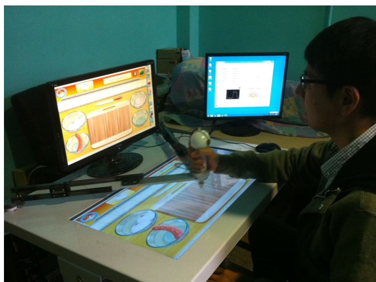
Figure.1 Upper limb rehabilitation robot integrated with video games
