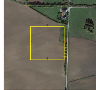
Figure 5: One GPS position (middle) with four 100 m deviations (up, down, left, right) and the yellow noise window.
