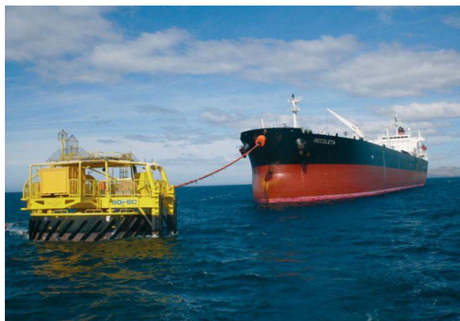
Figure 1-1 Tanker moored to an SPM system (SOFEC, 2009) [1]
