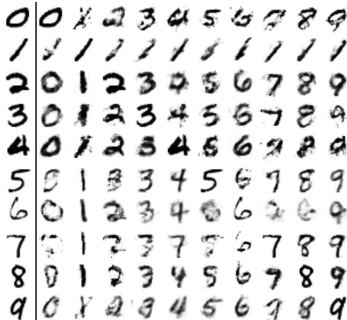
Figure 2: Images from MNIST dataset, along with their synthetic analogies generated by M2 [13] with the same inferred style ( z ), but with a changed label ( y ). In the left column are the original images, and each following column corresponds to analogies with labels 0-9. Note how the reconstructions on the diagonal match the original image the best.
