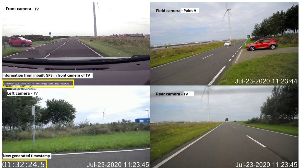
Figure 5.7: A still of combined video footage after video synchronisation
