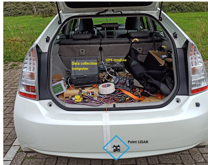
Figure 4.7: LiDAR, GPS and data collection devices in test vehicle
