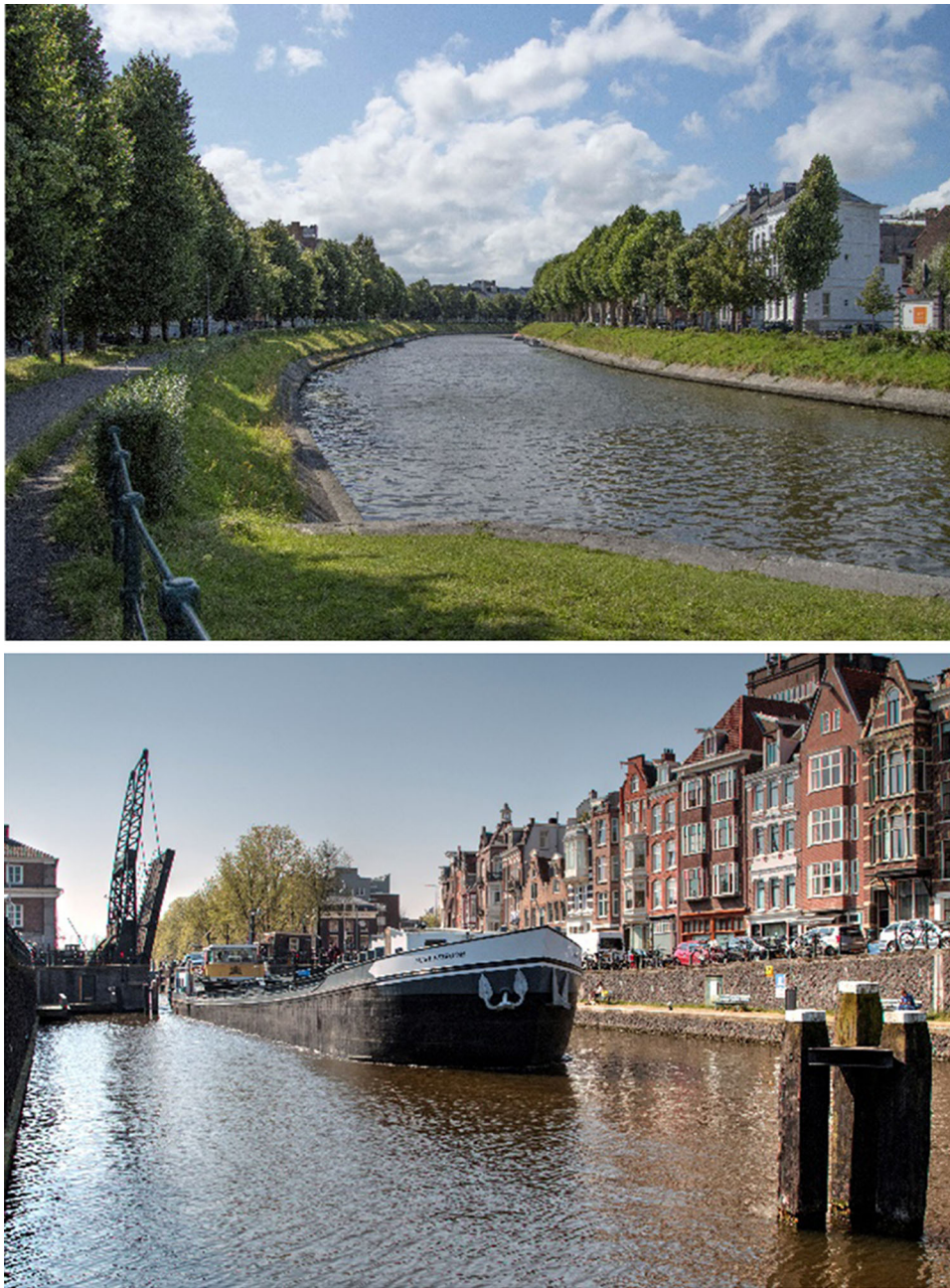
Fig. 2 Most canals and canalized rivers have vertical quay walls (bottom, Schippergracht in Amsterdam), some have sloping banks with hard bank protection (top, Coupure in Ghent). Pictures by Marc Brink
