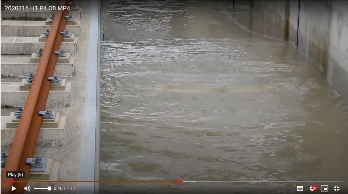
Figure 3.10: Unwanted behaviour during the experimental scale tests: Complete submersion 1
