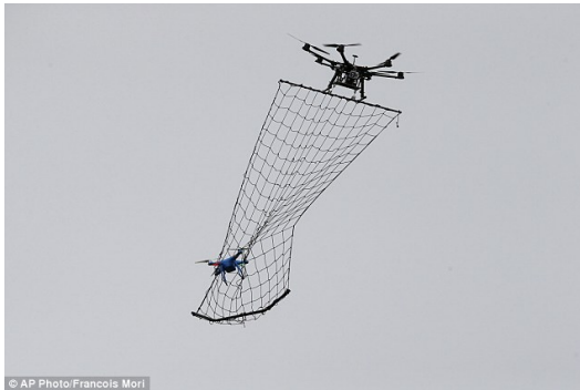
Figure 3.1: MPI-200 capturing a drone [27].
