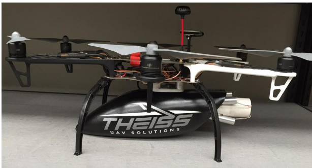
Figure 3.3: Theiss UAV's Excipio net gun, mounted on a hexacopter [52].
