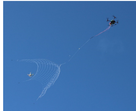
Figure 3.2: DroneCatcher capturing a drone [10].
