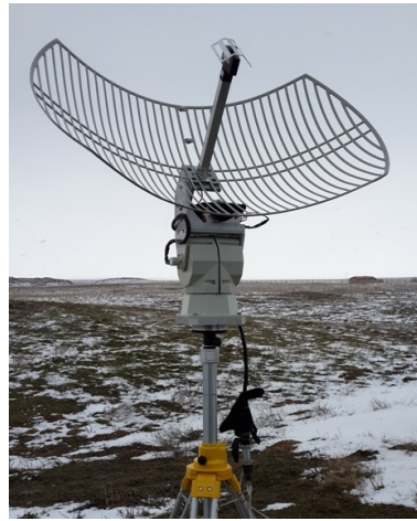
Figure 14.6: TUALLINK ground terminal antenna [54].
