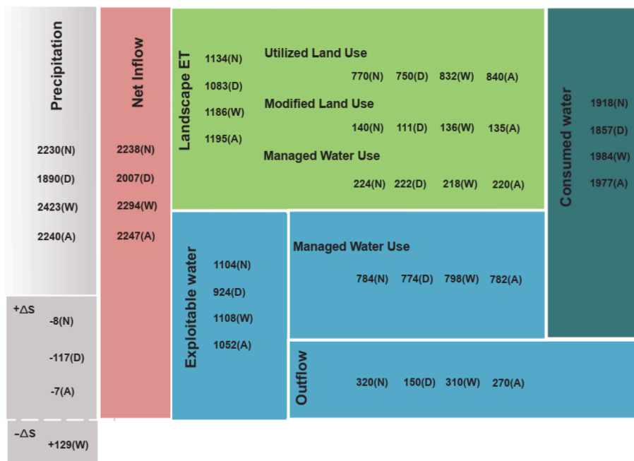
Fig. 5. WA + resource base sheet (MCM/year) for the time period of Oct 2010–Sep 2016
