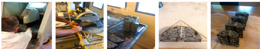
Figure 2. SCB test specimen cutting and marking process.
