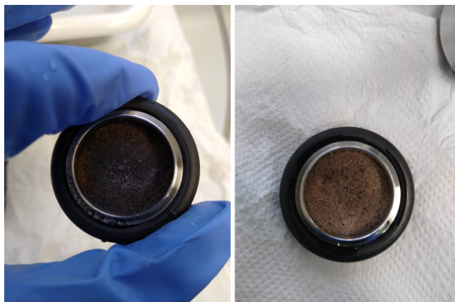
Figure 3.14: Difference in NP retention in porous tablet without (Left) and with citric acid (Right)
