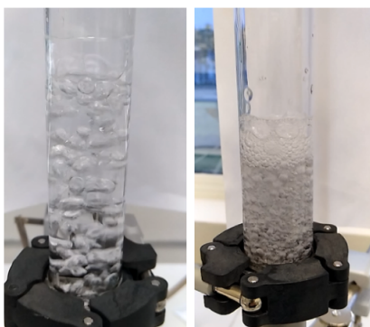
Figure 3.10: Difference in bubble formation without (Left) and with citric acid (Right)
