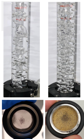
Figure 3.7: Difference in Bubble formation with mesh (Left) and with Bronze tablet (Right) (Reproduced from Striekwold)
