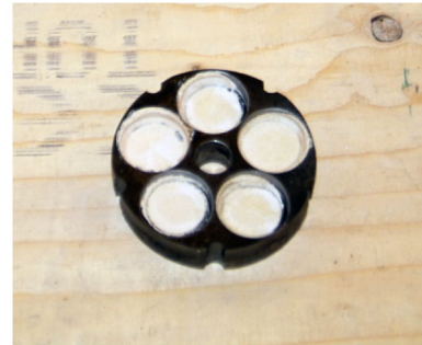
Fig. 11 Load introduction pre-study: endcap with Hilti-HIT after loading and disassembly
