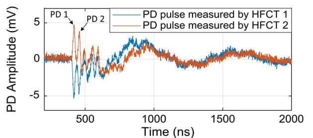
(b). TRPD pulses of two partial discharges in series at 108 kV<sub>rms</sub>.
