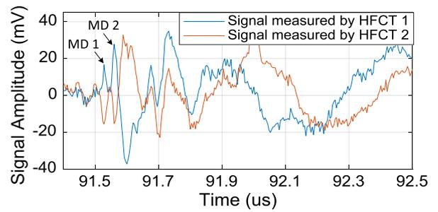
(a). TRPD pulses of MD1 and MD2 measured under impulse voltage.
