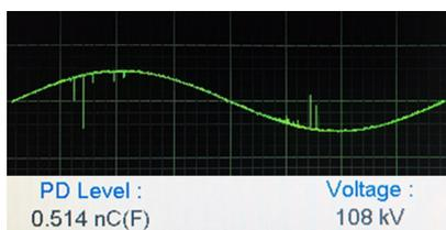
Fig. 14. Partial discharges at 108 kV<sub>rms</sub> measured by conventional method.
