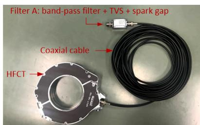
(a). Configuration of measuring system combined with HFCT, filter A and the connecting coaxial cable.
