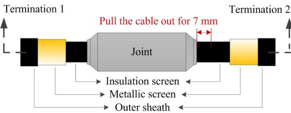
Fig. 3. HV cable joint and the artificial defect.
