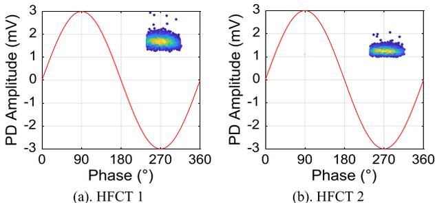
Fig. 10. PRPD patterns of corona discharges at termination 1.
