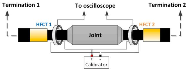
Fig. 8. Pulses simulated from the cable joint.
