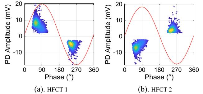
Fig. 12. PRPD patterns of partial discharges at 108 kV<sub>rms</sub>.
