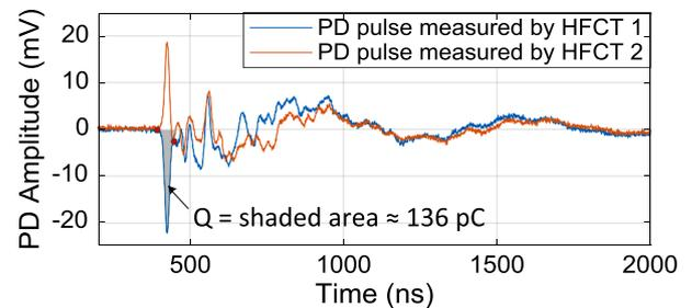
(a). TRPD pulses of one partial discharge at negative cycle of 108 kV<sub>rms</sub>.
