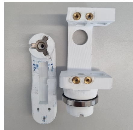
Figure 5.8: Picture of the components affected by the meltdown of one of the servos during the first test runs. On the left, it is clear how the melting ASA allowed the inserts to slip out of the reserved holes and the damage at the base of the servo's wiring. On the right, the damage to the other component is more clear, with the huts designed for the servo metallic heads fatally worn out.
