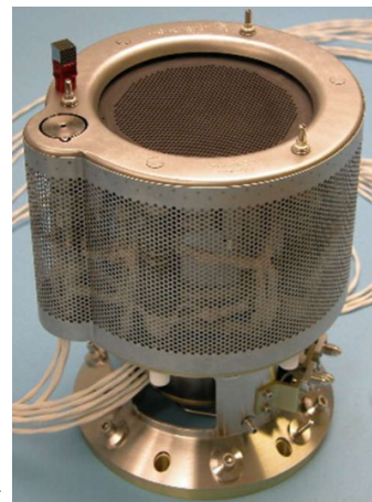
Figure 6.10: The Qinetiq T5 ion thruster [5]
