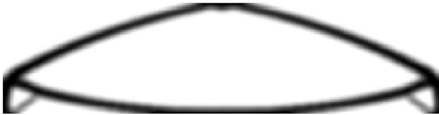
Fig. 7 Beam minimum compliance topology design with QP update ( f = 0.16/4 ): k = 335 , f_0 = 6.650 , V = 0.16 , B\&W = 0.99
