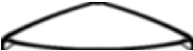
Fig. 8 Beam minimum compliance topology design with QP update ( f = 0.16/2 ): k = 451 , f_0 = 11.84 , V = 0.16 , B\&W = 0.99
