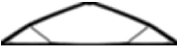
Fig. 9 Beam minimum compliance topology design with QP update ( f = 0.16 ): k = 244 , f_0 = 25.28 , V = 0.16 , B\&W = 0.99
