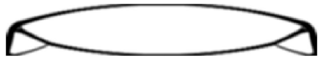
Fig. 1 Self-weight MBB beam minimum compliance topology design with QP update: k = 132 , f_0 = 6.194 , V = 0.14 , B\&W = 0.96
