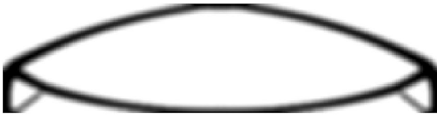
Fig. 6 Beam minimum compliance topology design with QP update ( f = 0.16/10 ): k = 160 , f_0 = 4.167 , V = 0.16 , B\&W = 0.98
