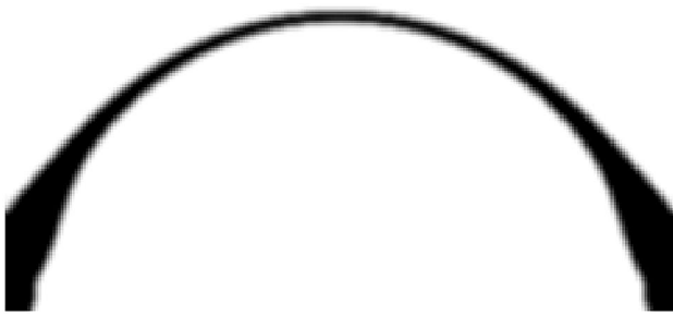
Fig. 2 Self-weight arch minimum compliance topology design: k = 171 , f_0 = 0.1261 , V = 0.10 , B\&W = 0.99
