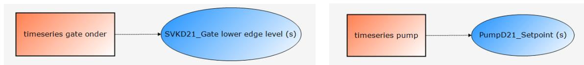
Figure D.7: SOBEK control groups of the storm surge barrier and pumping station
