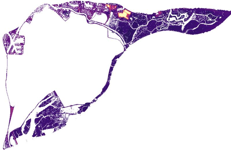
Figure A.2: Digital Terrain Model map of the flood prone areas not protected by flood defenses
