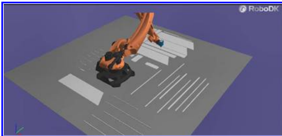
Fig. 5 RoboDK software package for manufacturing simulation. On the floor the different wing panels and stringers which needed to be drilled.
